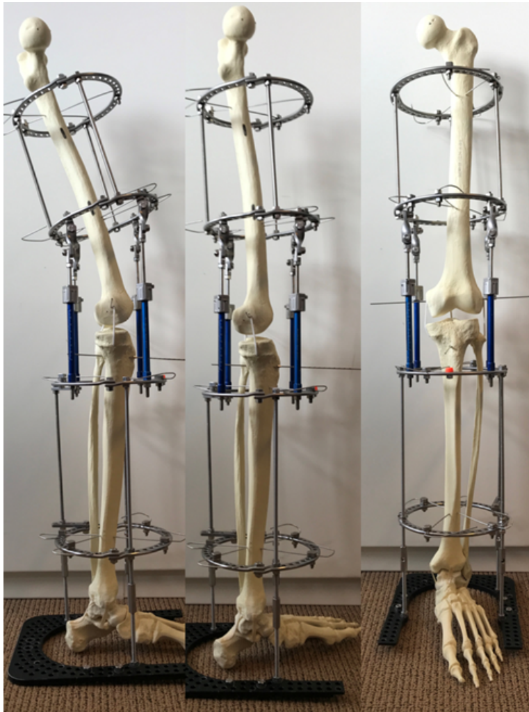
Figure 10: Different positions of the sawbone model. The left image shows a flexed position. The centre image shows a fully extended position. The right image shows the antero-posterior plane of the model, leg rotation means rotating from this plane and position.
