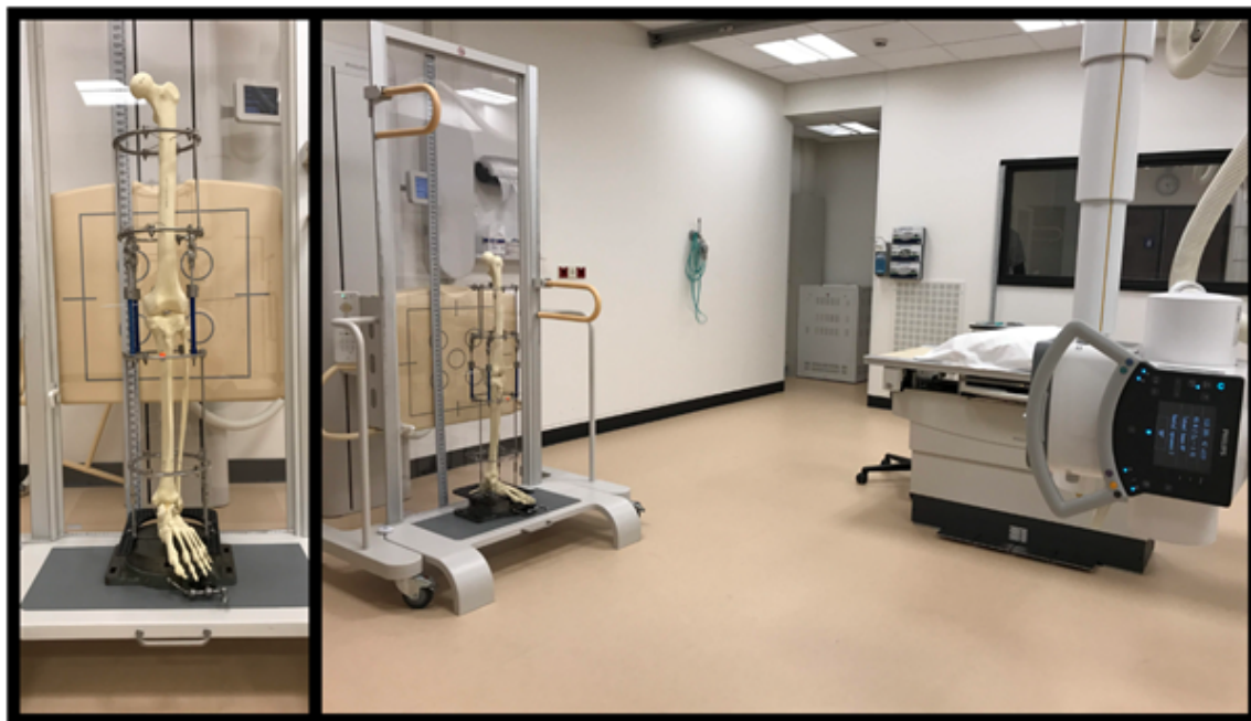
Figure 7: Measurement setup in the projection radiography room, with the Bucky system Philips DigitalDiagnost v4.0.
