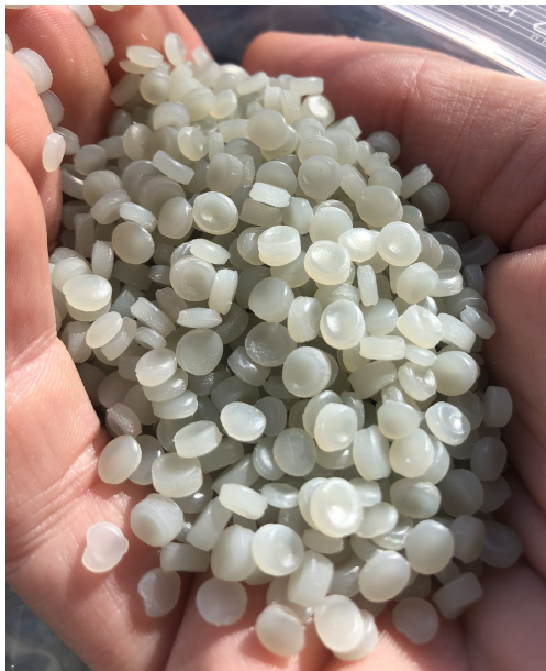
Figure 6: End product in the form of LDPE pellets. Shown in picture are natural pellets.
