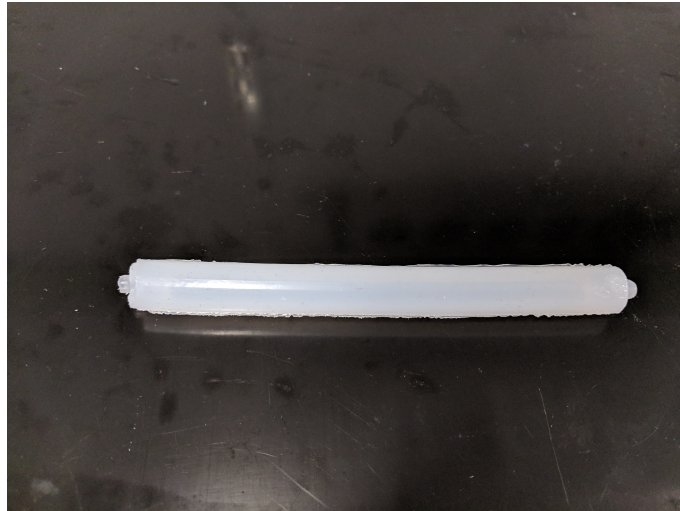
Figure 4.5: Silicon bladder after removal from the mold.
