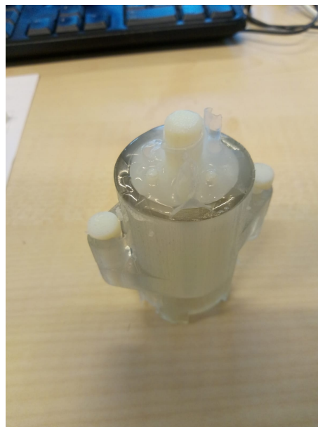
Figure 5: Result of the first layer of EcoFlex 0030 inside the module mould. The metal bars already have been taken out.
