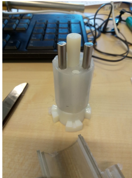
Figure 7: Re-assembled module part to prepare for the pouring of DragonSkin 10. The cover is placed on the top of the white base-connector, creating an extra space above to pour the material in.
