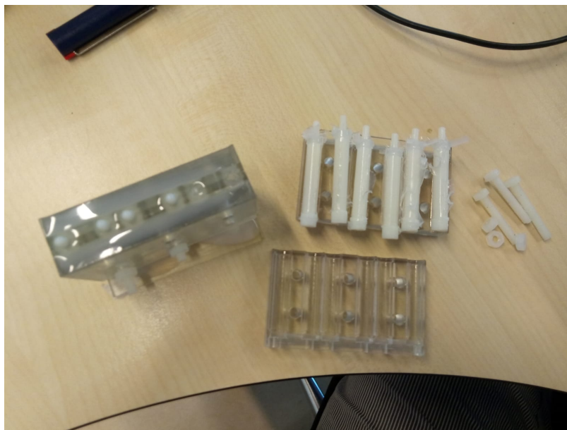
Figure 3: Image showing the poured mould (left) and the resulting chambers (right), together with a view on the inside of the mould and its fixation material (below and right). Process designed by Jan Lenssen (Lenssen, 2019).
