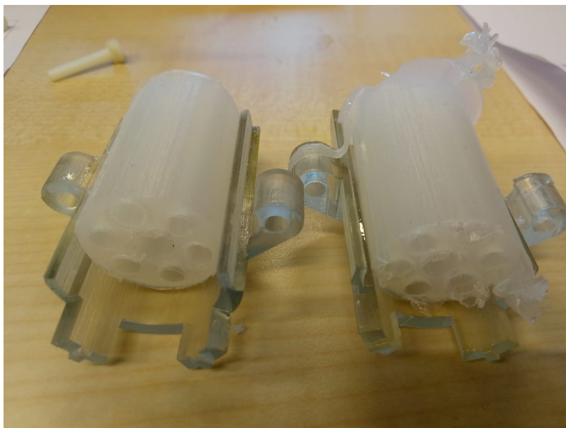
Figure 6: Bottom mould of the endoscope module fabrication process. Design based on the design of Jan Lenssen (Lenssen, 2019), adjusted to fit the use of extra holes in the module.
