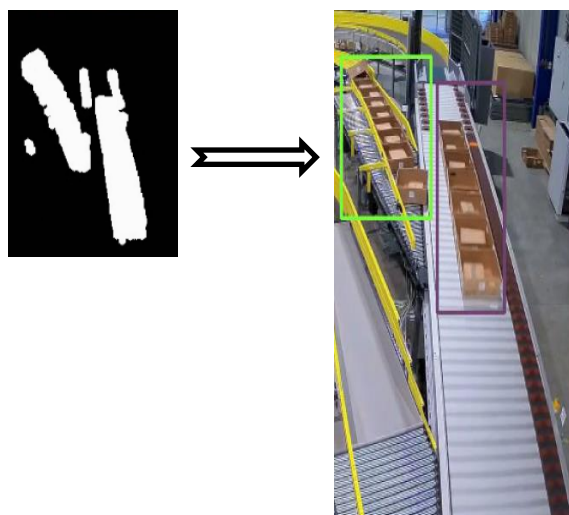
Figure 45– Foreground extraction using Background subtraction [123]
