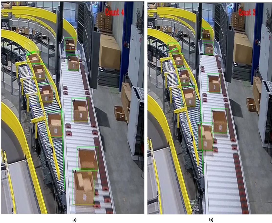
Figure 55- No Jam videos a) Tracking in the Nth frame and the corresponding count in the OFZ b) Tracking in the N+1 frame and corresponding count in the OFZ where one TSU (ID=1) has moved away from the exit line of the OFZ. The track IDs are sustained (1,3,5,7).
