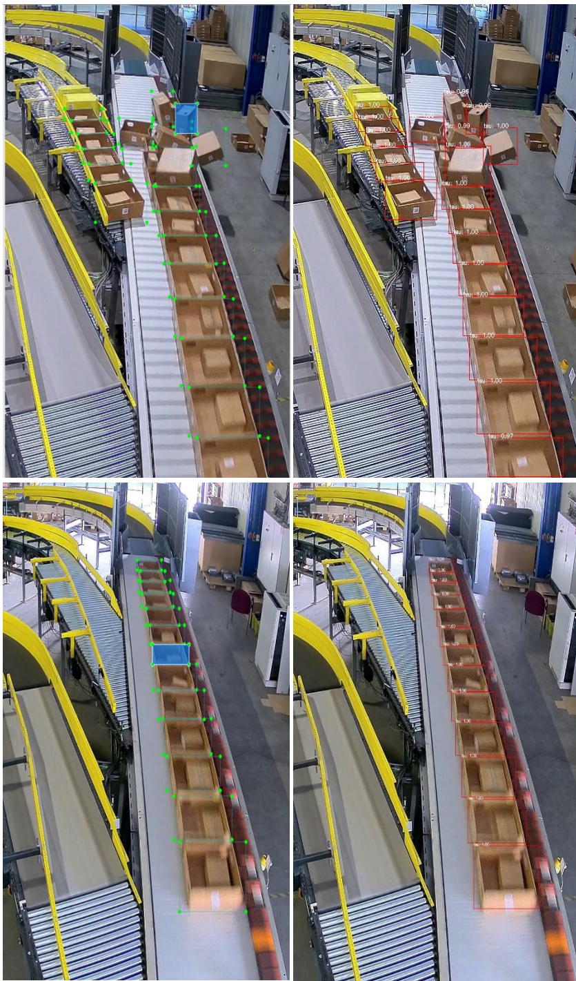
Figure 53 – a)& b) Results from the jam and no jam footages with different lighting conditions with ground truth (left) and corresponding prediction (right)
