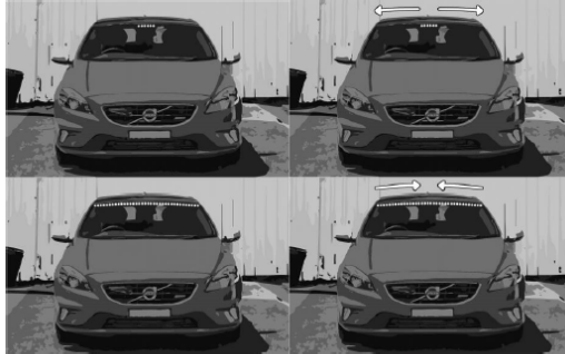
Figure 38. Top left: AD mode. Top right: Yielding. Bottom left: Resting. Bottom right: Starting.
