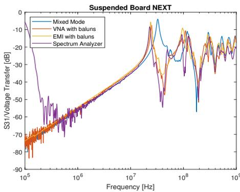
Fig. 9: Suspended Board NEXT measurement
