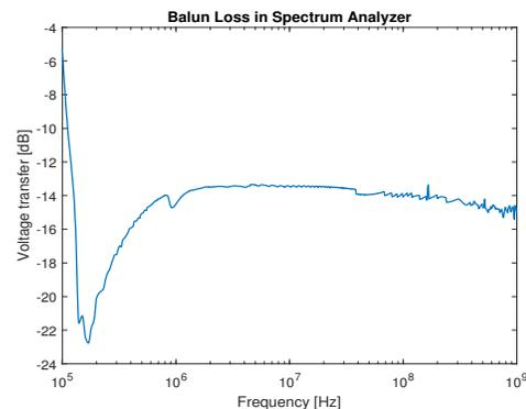
Fig. 15: Balun Effect in the Spectrum Analyzer
