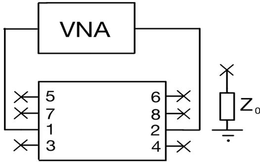
Fig. 4: Setup for single-ended measurements
