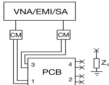
Fig. 3: Setup for balanced measurements
