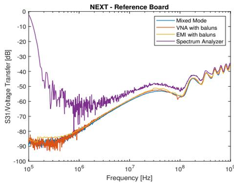
Fig. 5: Reference Board NEXT measurements
