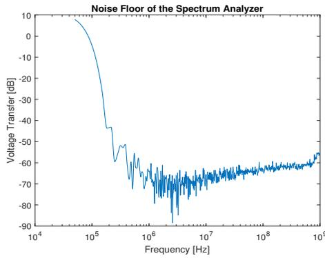
Fig. 16: Noise Floor of the Spectrum Analyzer
