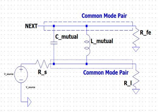
Fig. 1: The simplified model for common-mode NEXT
