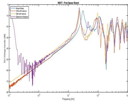
Fig. 7: Free Space Board NEXT measurements
