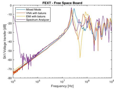
Fig. 11: Free Space Board FEXT measurement
