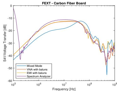
Fig. 12: Carbon Fiber Board FEXT measurement
