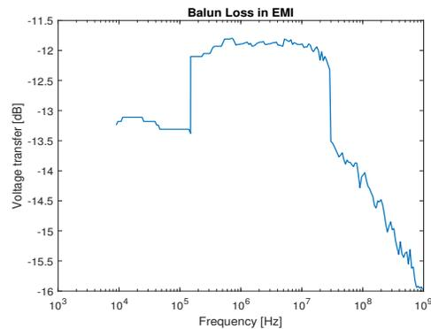
Fig. 14: CM balun loss measurement
