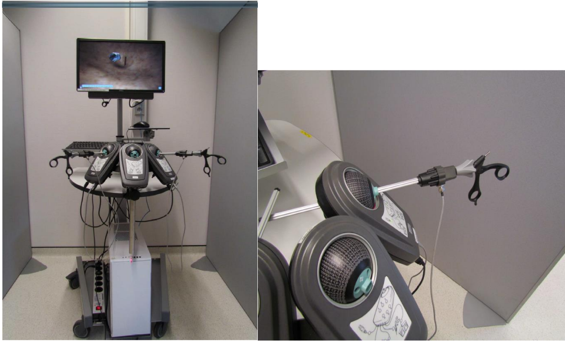
Figure 2 - Setup of the Lapsim: Three SimBall-modules, as well as the desktop computer and LC-display. The table can be adjusted in height to allow for a comfortable posture during task performance.
