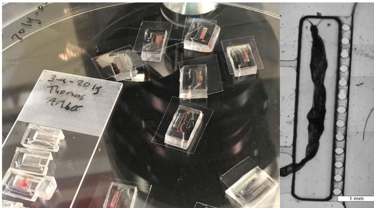
FIGURE 23. CHIPS ARE APPROXIMATELY 12MM BY 6MM. THE PDMS CHIPS ARE LOADED WITH EPIDIDYMAL TUBULES ORIGINATING FROM THE CORPUS SEGMENT AND ARE CLOSED WITH PCR TAPE. THE RIGHT IMAGE SHOWS A PIECE OF EPIDIDYMAL TUBULE INSIDE A CHIP AND CONFINED IN THE CULTURE CHAMBER WITH THE MICROCHANNEL BARRIER ON THE RIGHT.
