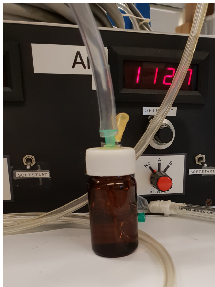
Figure 9: The purging setup: green cap = inlet, yellow cap = outlet
