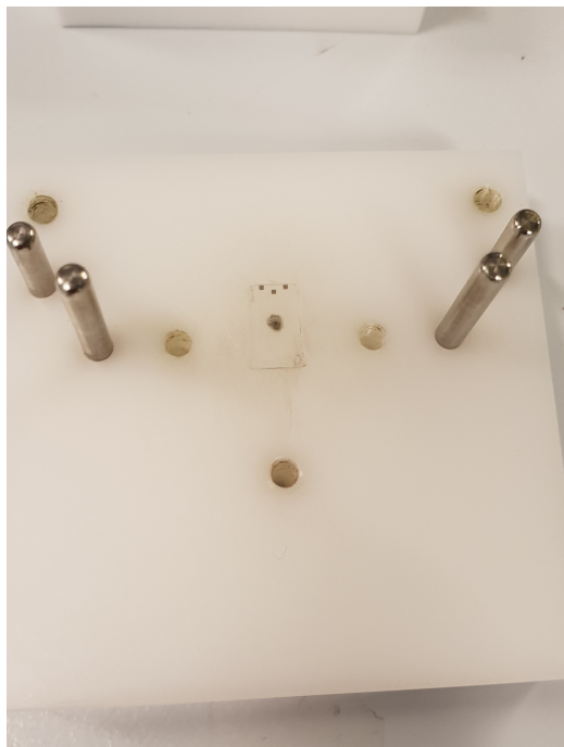
(a) Teflon base, with a RuOx chip mounted
