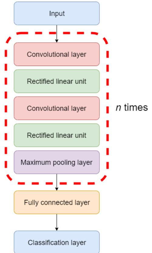
Figure 4.5: Architecture of CNN. In experiment 1a the value of  $n$  is found.
