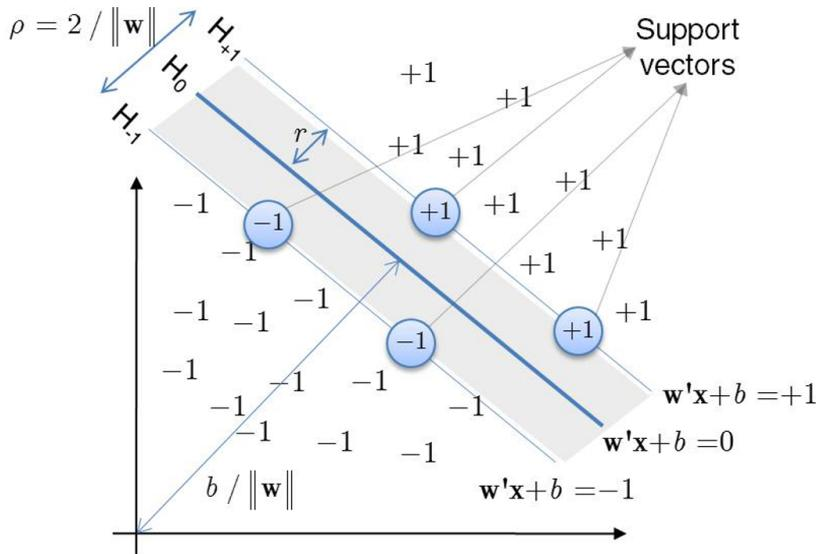
Figure 3.2: Schematic representation of an SVM in a two-dimensional space [29]
