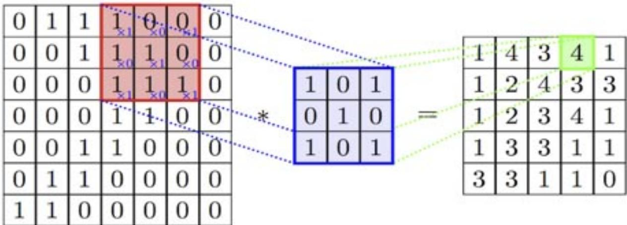
Figure 3.4: The working of a convolution in a convolutional layer. On the left, the input is shown. In the middle, the kernel (blue) is shown and on the right, the result is shown. In this example, the kernel represent a cross, because the ones are in all the corners and in the middle and the spaces in between are filled with zeros. [31]
