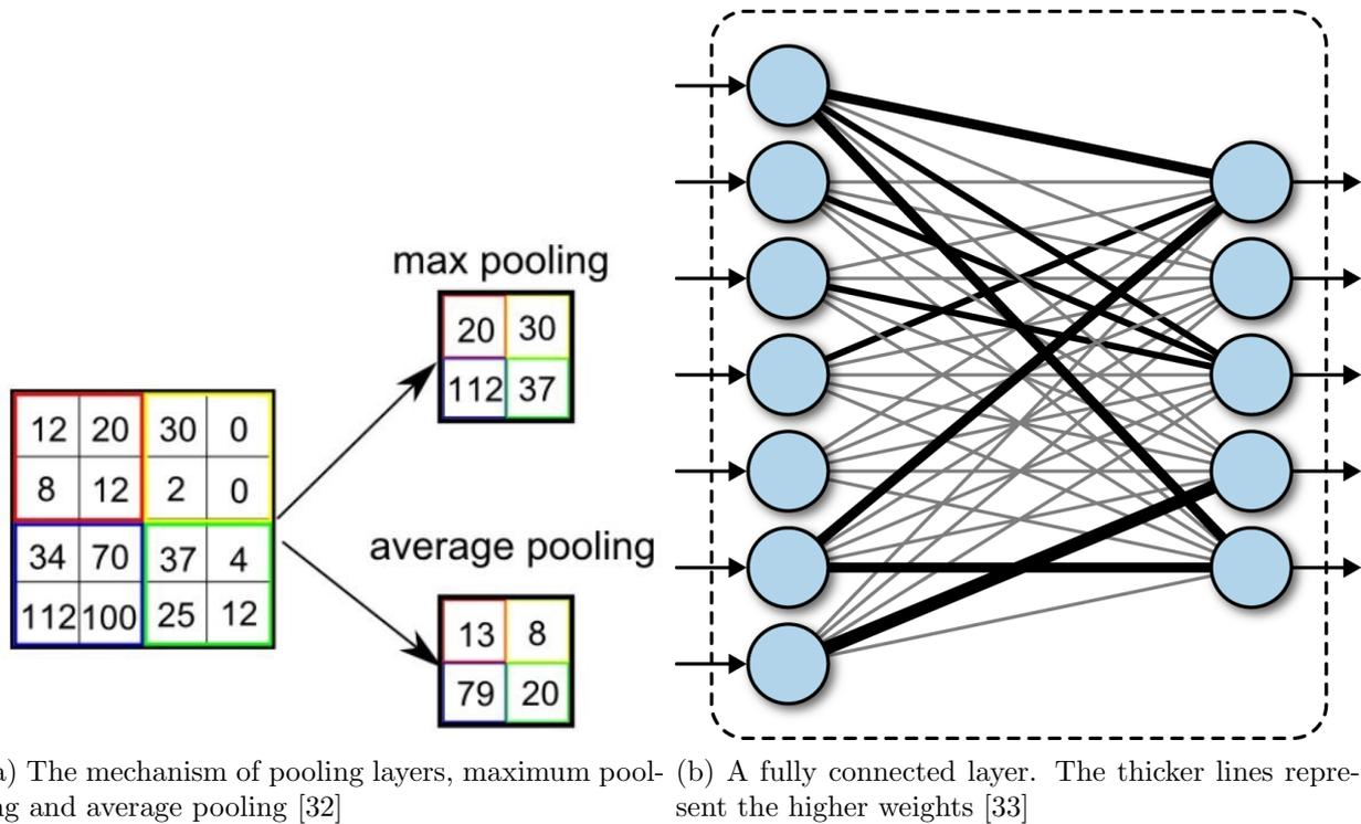
Figure 3.5: Explanation of two layers in a CNN.
