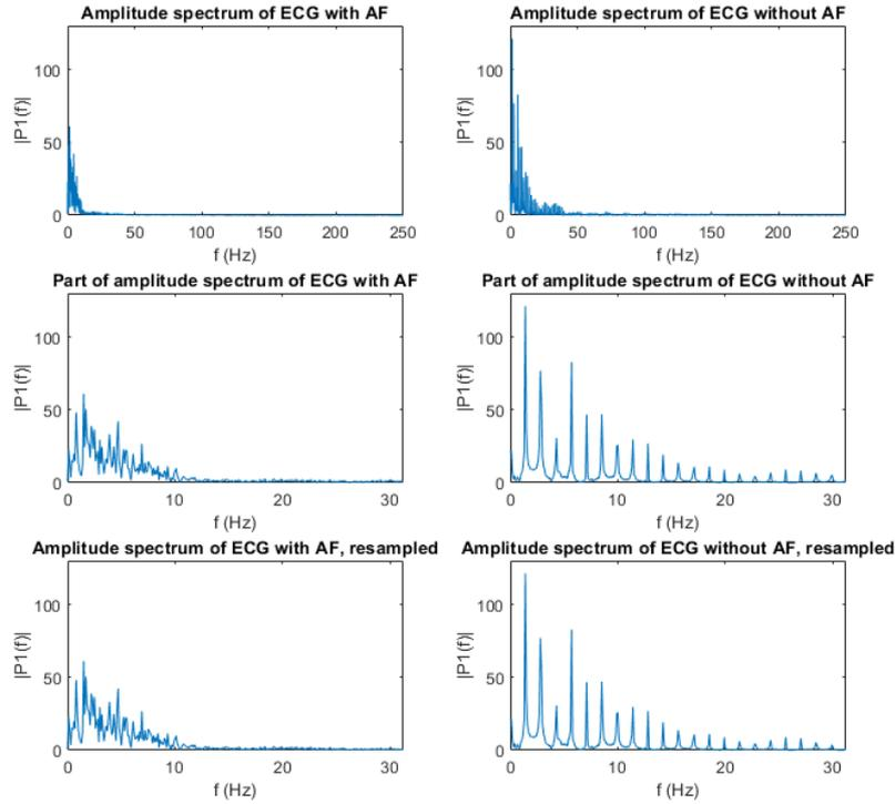
Figure 4.4: Amplitude spectrum of two original signals with the amplitude spectrum of their resampled signals as a comparison. It can be seen that the frequencies which are present in the original signals are also present in the resampled signals.
