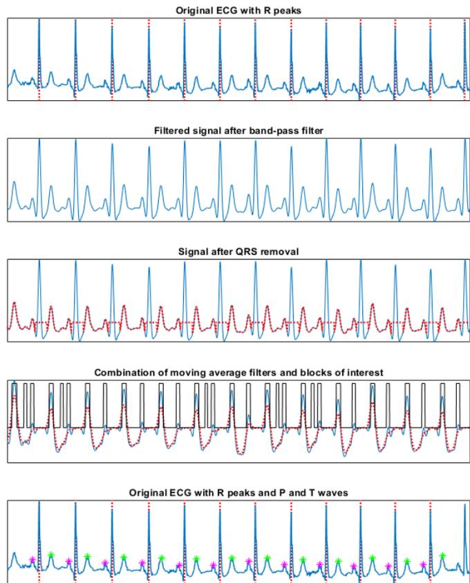
Figure 5.4: Different steps of the P and T wave detection algorithm. The last R peak is ignored, because it is too close to the border.
