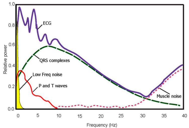
Figure 5.3: Frequencies which are present in the ECG signal [51]
