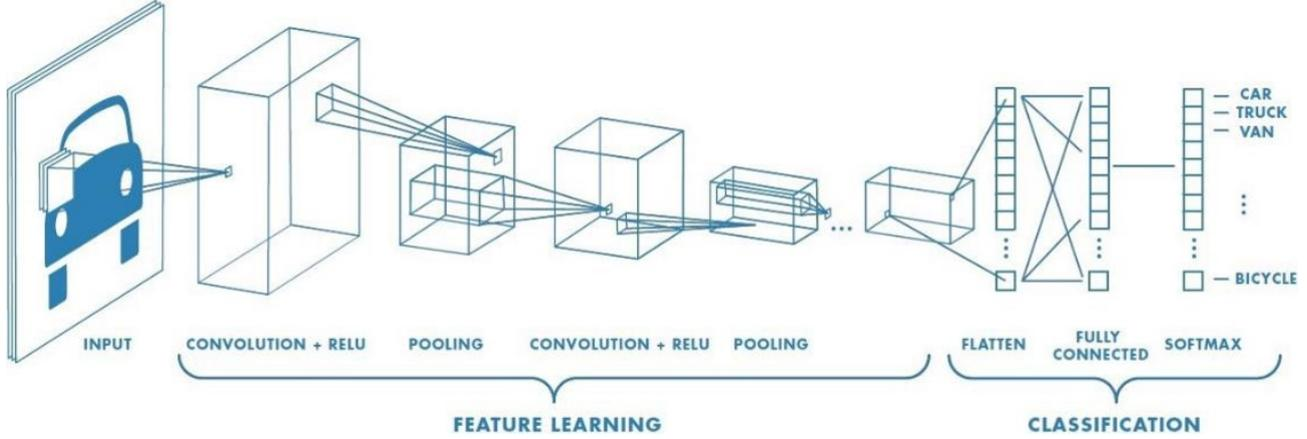
Figure 3.3: The structure of a CNN [30]
