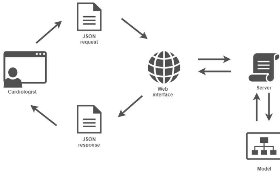
Figure 6.5: The technical details of the REST API service. The JSON request contains the ECG and the JSON response contains the prediction score.
