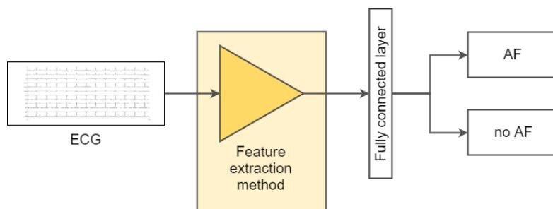
Figure 4.1: Set-up of the method used in experiment 1 of this chapter. An 8-leads ECG is used to detect AF or no AF. Here, the feature extraction method which is used is a CNN.
