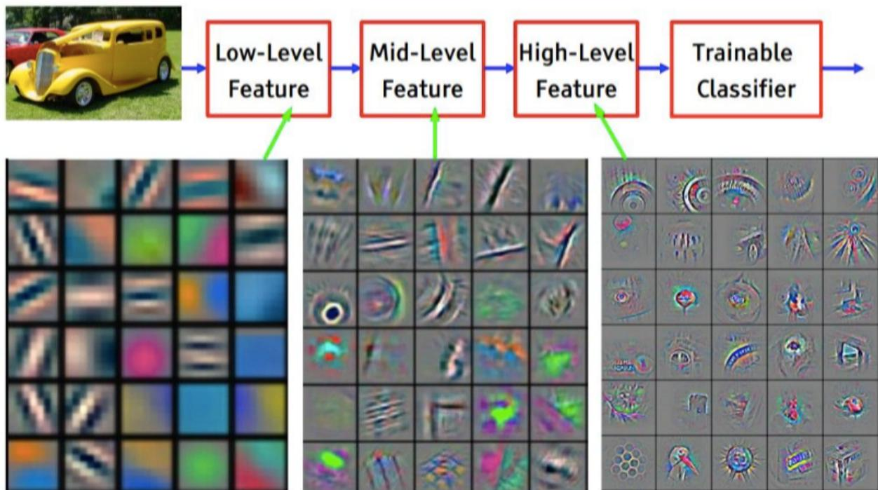
Figure 3.7: Features in different layers in a CNN [35]
