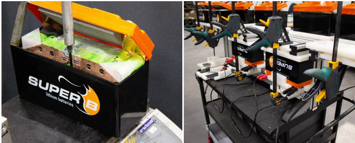
Figure 2.7 - Potting (left) and the harden process (right) for the Starter battery
