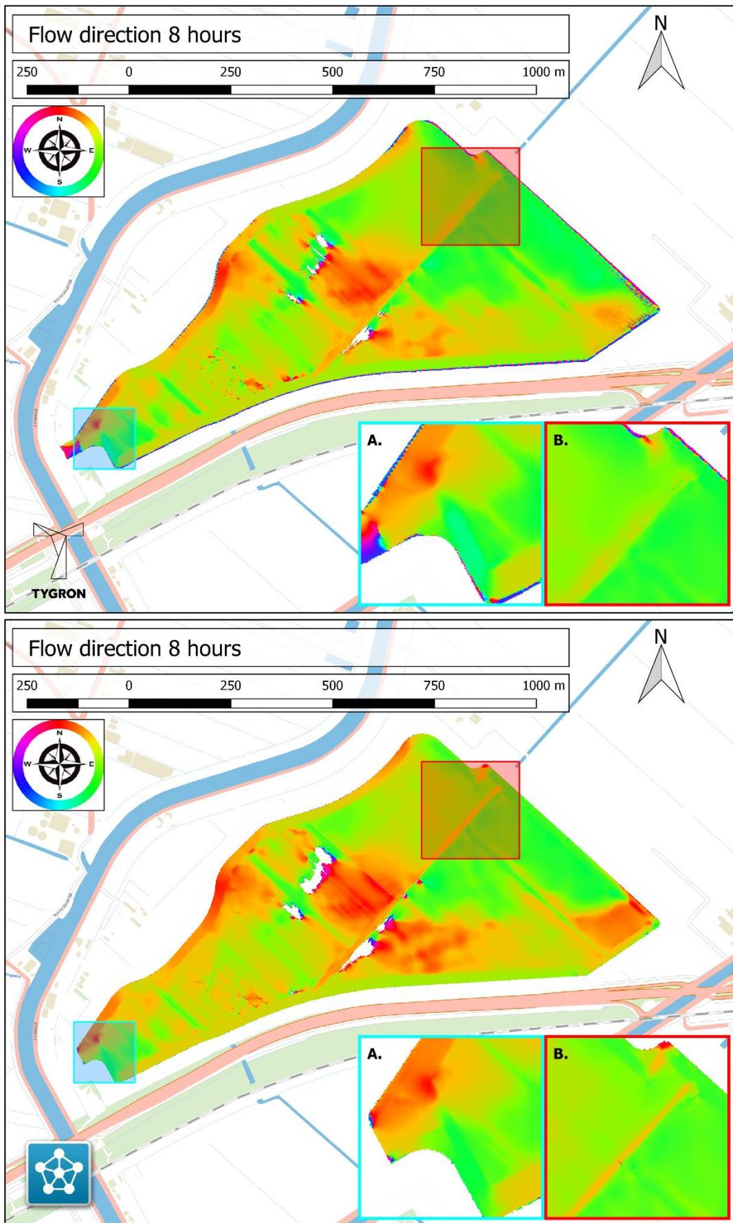
Figure A.9: Flow direction at 8 hours for Tygron (top) and Delft3D (bottom).
