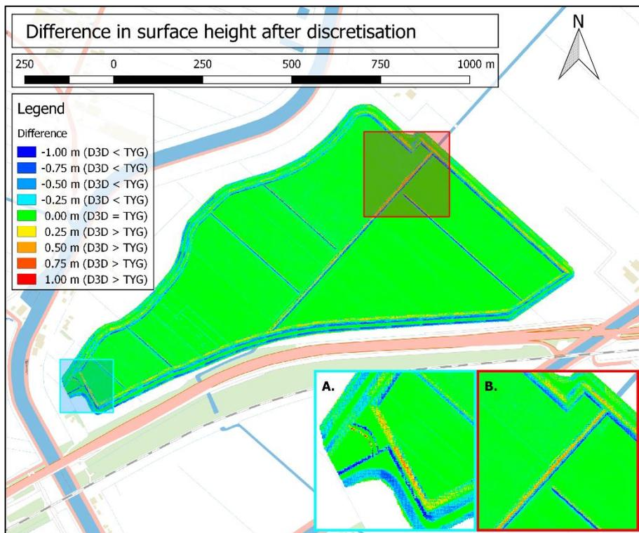
Figure 5.3: Difference in surface height after discretization of bathymetry to the grid.
