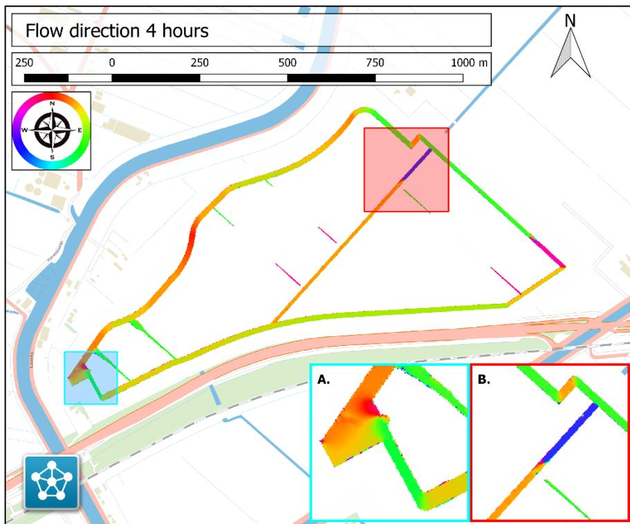
Figure 5.14: Flow direction at 4 hours for Delft3D.
