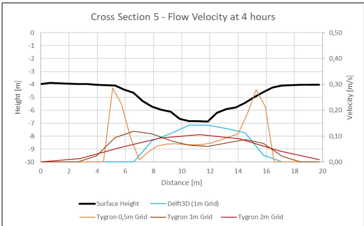
Figure B.5: Difference in flow velocity with different sized grids in Tygron.
