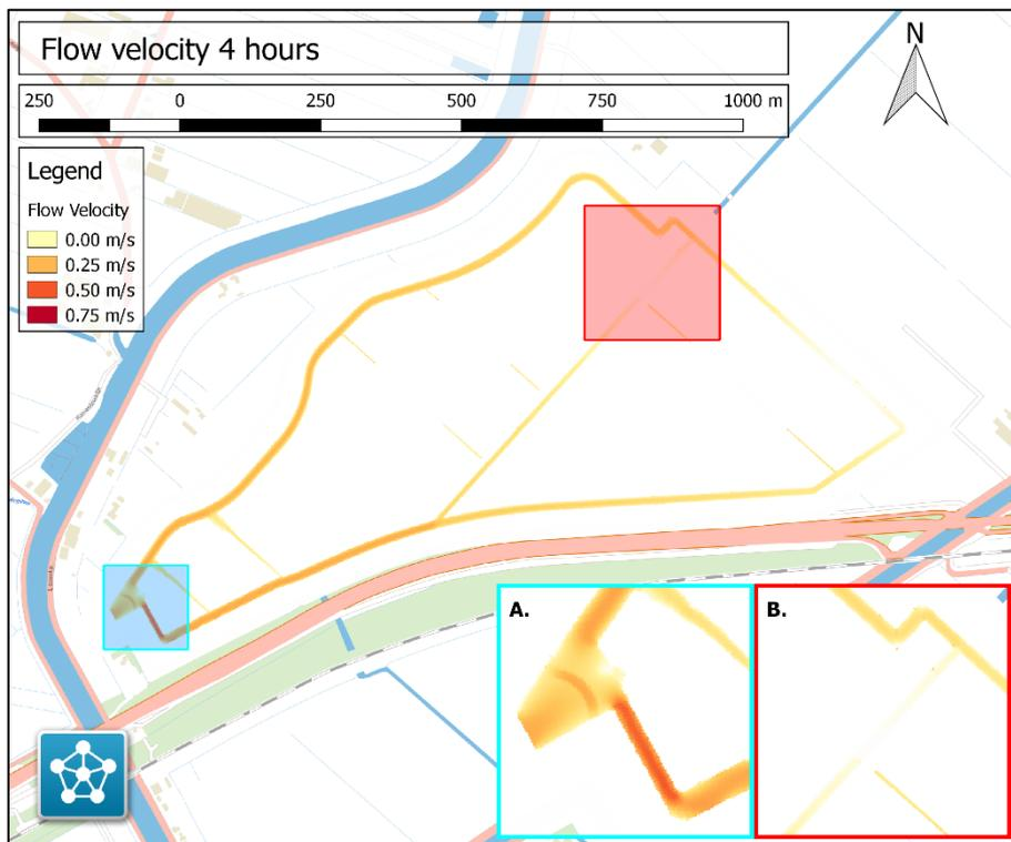
Figure 5.5: Flow velocity at 4 hours for Delft3D.
