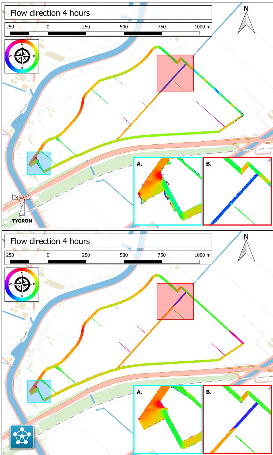
Figure A.8: Flow direction at 4 hours for Tygron (top) and Delft3D (bottom).
