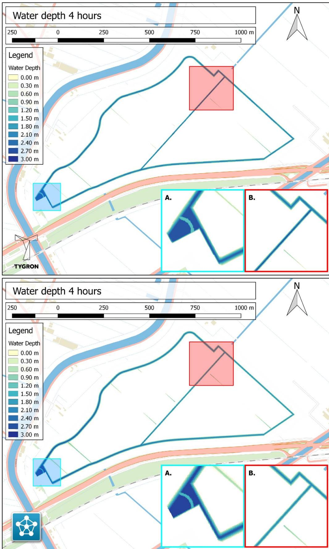
Figure A.2: Water depth at 4 hours for Tygron (top) and Delft3D (bottom).
