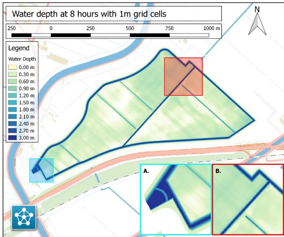
Figure C.5: Water depth at 8 hours with 1 meter grid cells.
