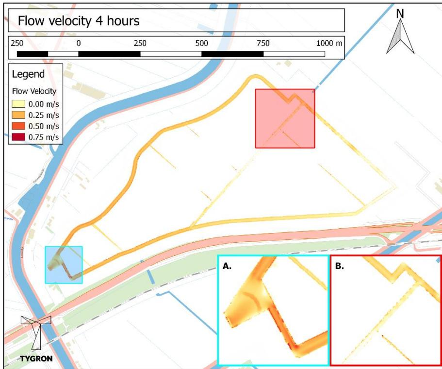
Figure 5.4: Flow velocity at 4 hours for Tygron.
