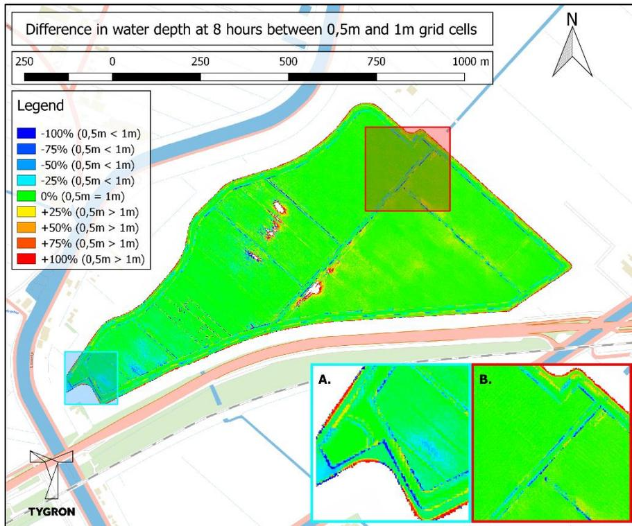
Figure B.7: Difference in water depth at 8 hours between 0,5m grid cells and 1m grid cells in percentages.
