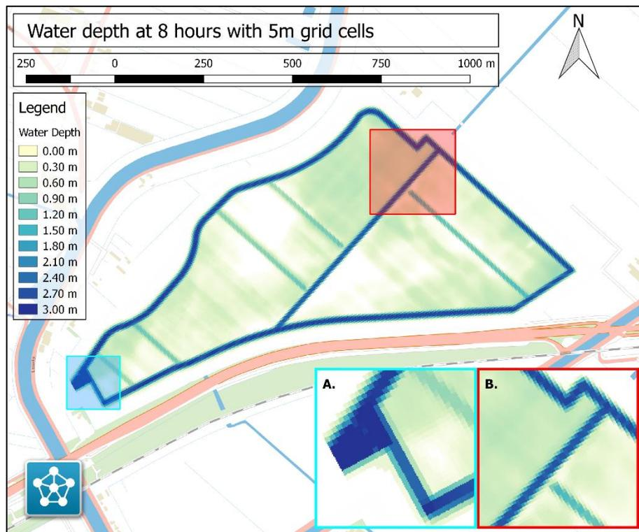
Figure C.6: Water depth at 8 hours with 5 meter grid cells.
