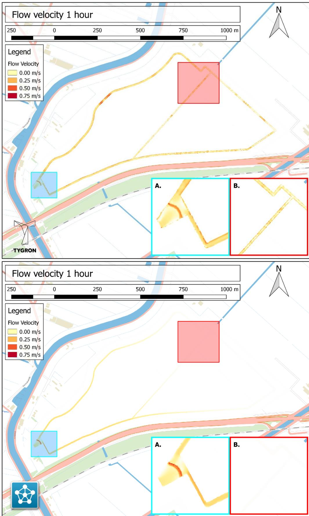
Figure A.4: Flow velocity at 1 hour for Tygron (top) and Delft3D (bottom).
