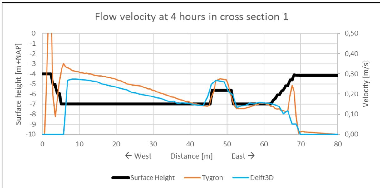
Figure 5.9: Flow velocity at 4 hours in cross section 1. (Surface height on left axis. Tygron and Delft3D flow velocities on right axis).
