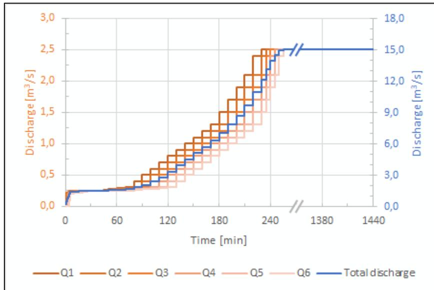
Figure 4.2: Inflow discharge in Tygron, with individual inlet points (Q1-Q6) on left axis and the total discharge on right axis.
