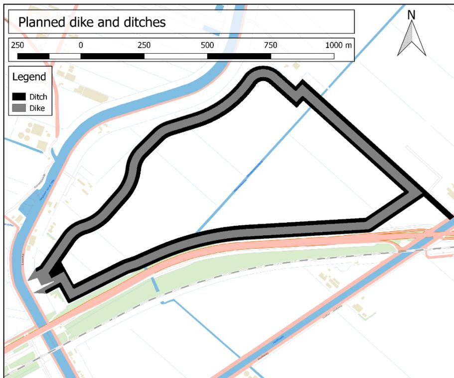
Figure 3.2: Planned dike and ditches in the case area
