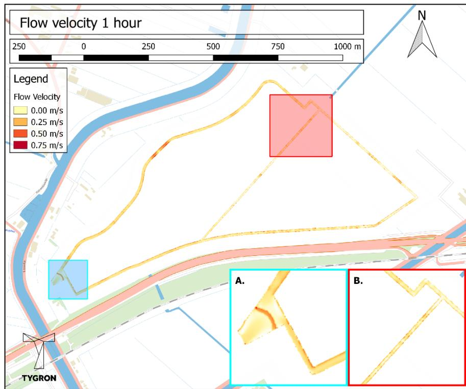
Figure 5.11: Flow velocity at 1 hour for Tygron.
