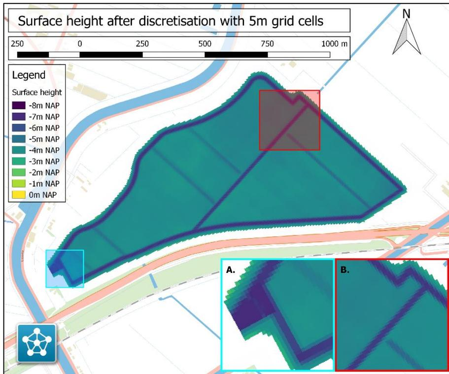
Figure C.2: Surface height after discretization with 5 meter grid cells.
