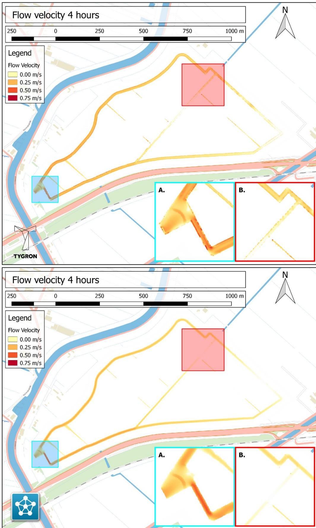
Figure A.5: Flow velocity at 4 hours for Tygron (top) and Delft3D (bottom).
