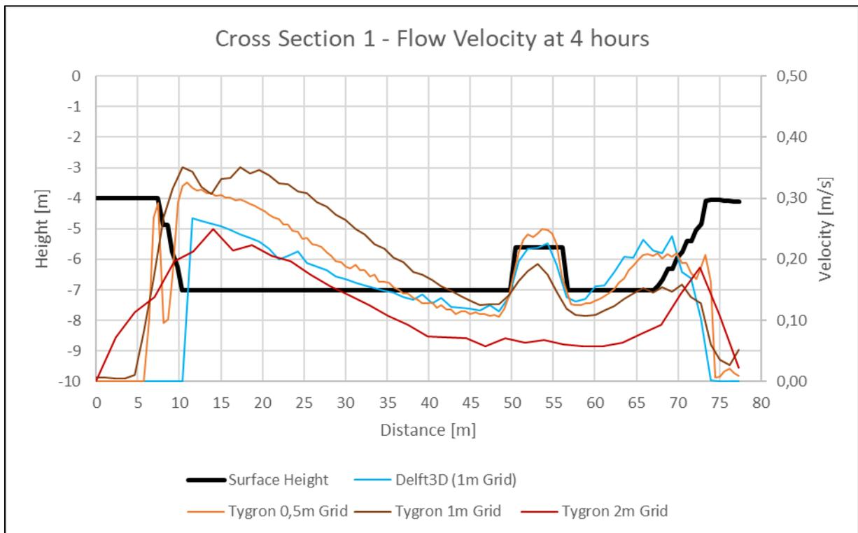
**Figure B.1: Difference in flow velocity with different sized grids in Tygron.**
