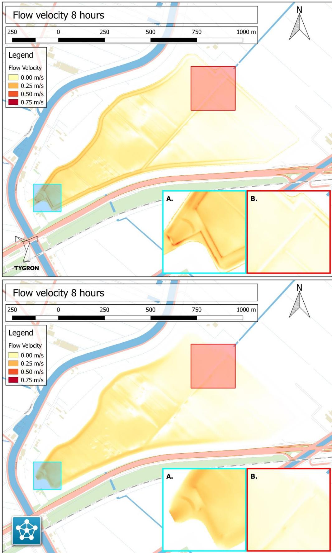
Figure A.6: Flow velocity at 8 hours for Tygron (top) and Delft3D (bottom).
