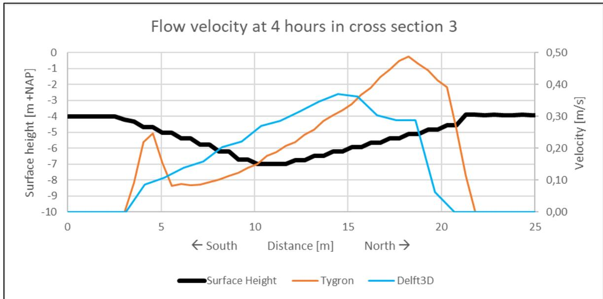
Figure 5.6: Flow velocity at 4 hours in cross section 3. (Surface height on left axis. Tygron and Delft3D flow velocities on right axis).
