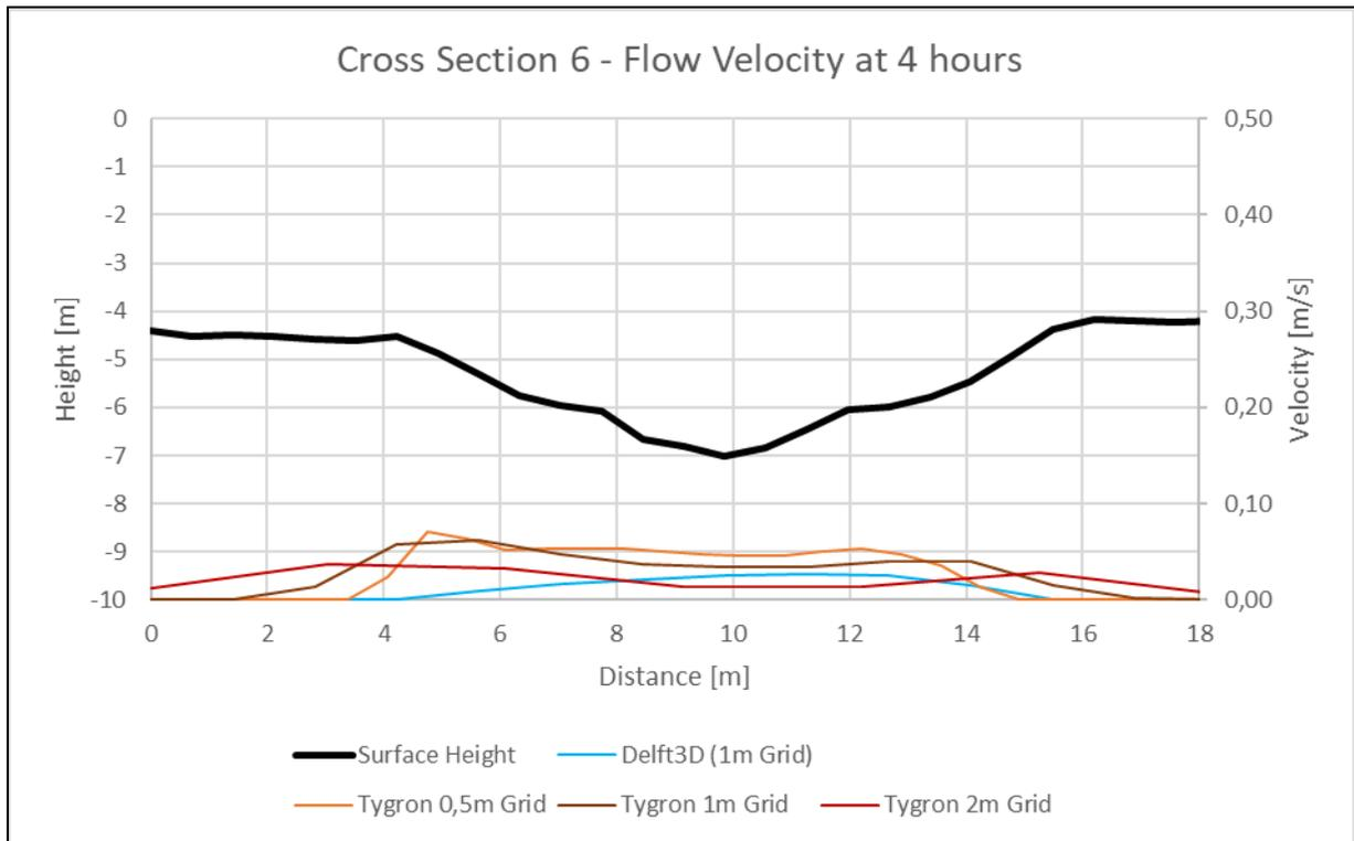
Figure B.6: Difference in flow velocity with different sized grids in Tygron.
