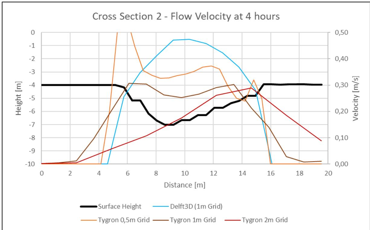
Figure B.2: Difference in flow velocity with different sized grids in Tygron.
