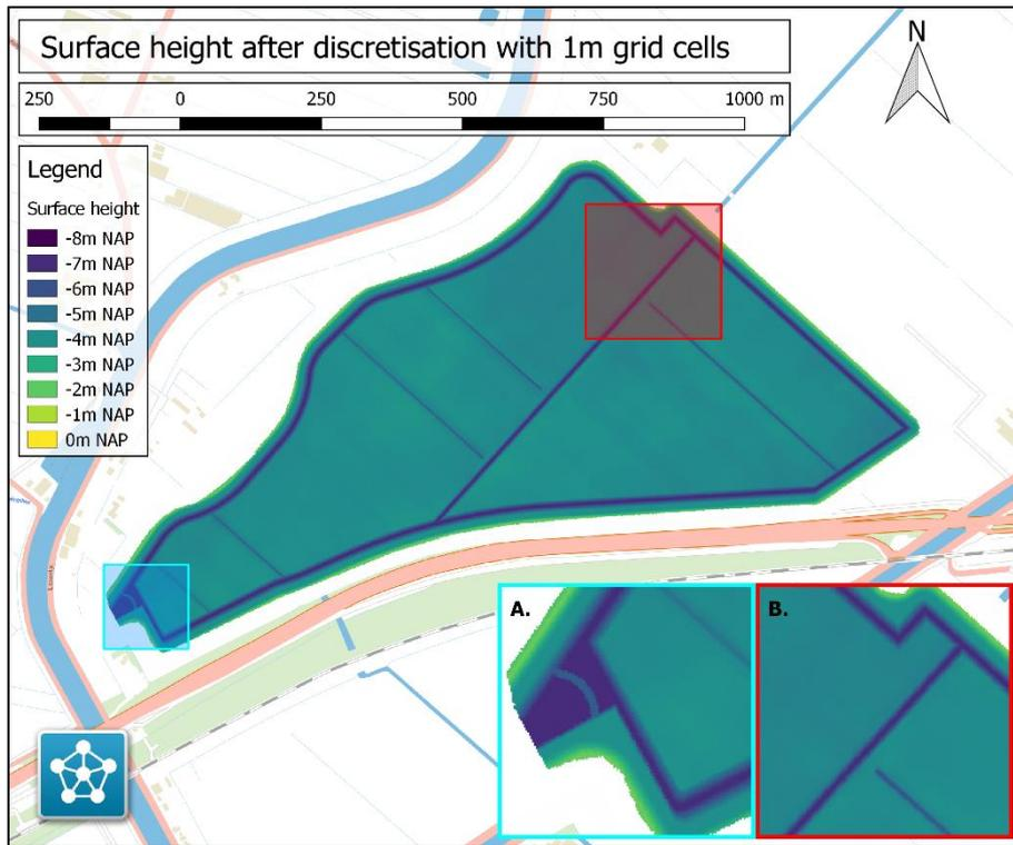
Figure C.1: Surface height after discretization with 1 meter grid cells.
