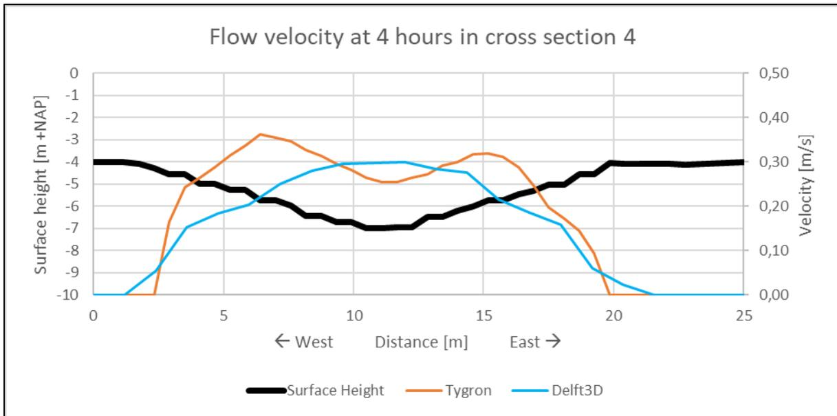
Figure 5.8: Flow velocity at 4 hours in cross section 4. (Surface height on left axis. Tygron and Delft3D flow velocities on right axis).
