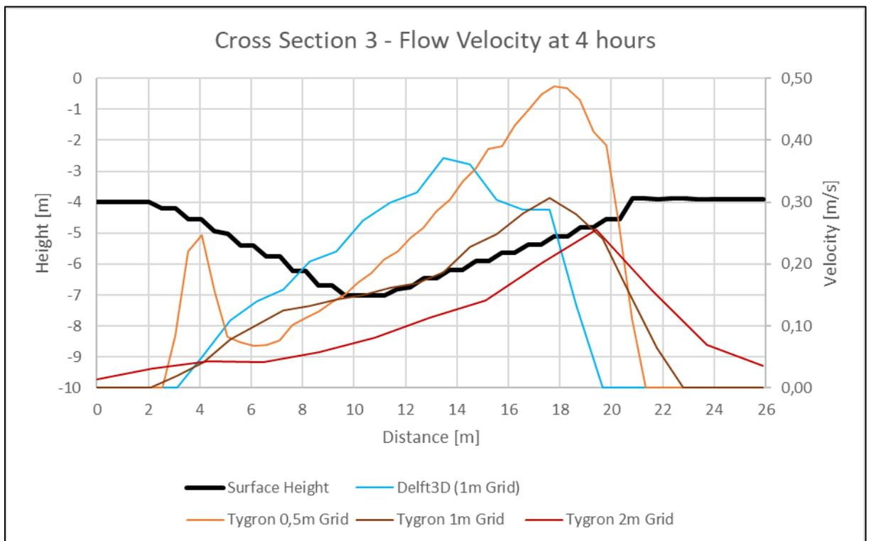
Figure B.3: Difference in flow velocity with different sized grids in Tygron.
