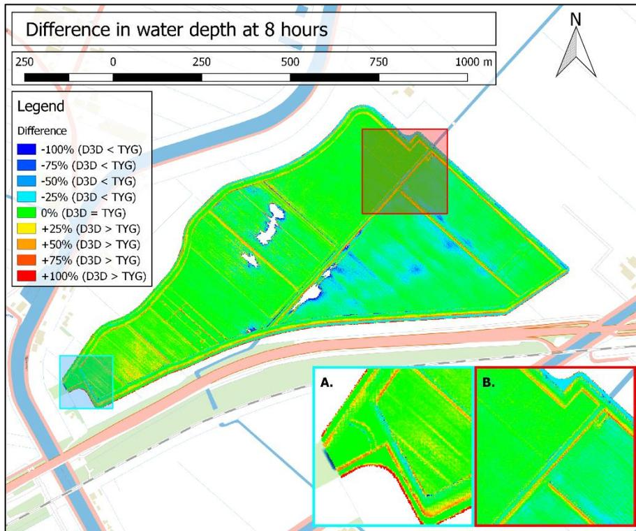
Figure 5.2: Difference in water depth between Tygron and Delft3D at 8 hours.
