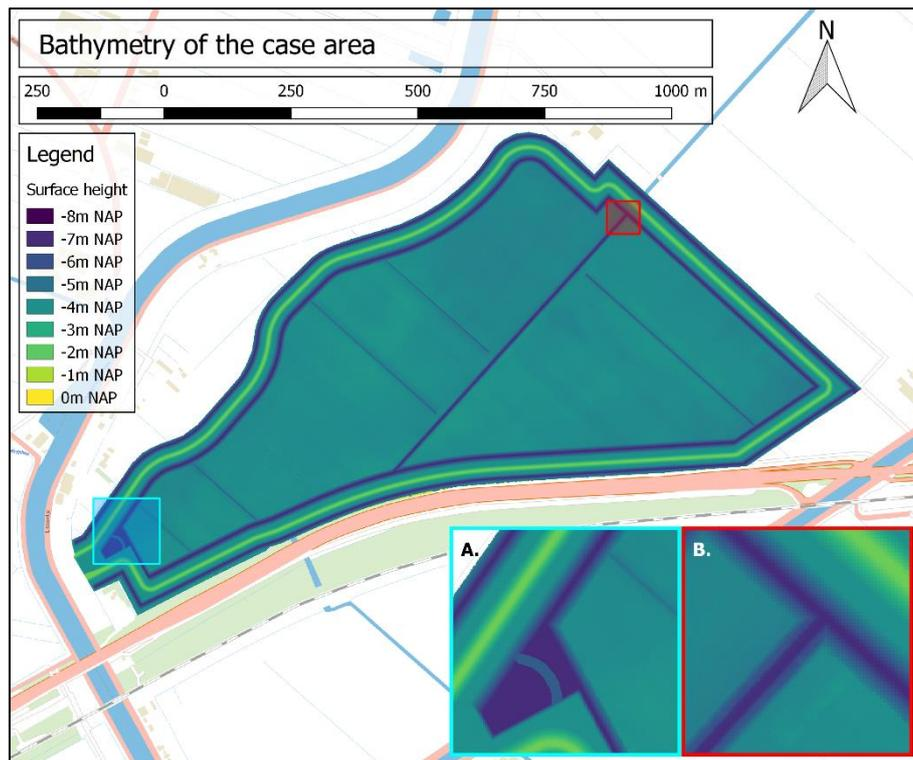
Figure 3.3: Bathymetry of the case area. (A: The inlet location with installed weir, B: Connection between the already existing and the installed ditch)
