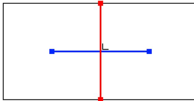
Figure 4.4: Grid orthogonality in a structured grid.
