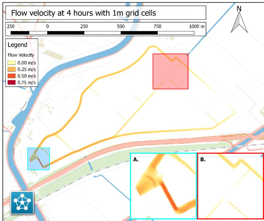
Figure C.3: Flow velocity at 4 hours with 1 meter grid cells.
