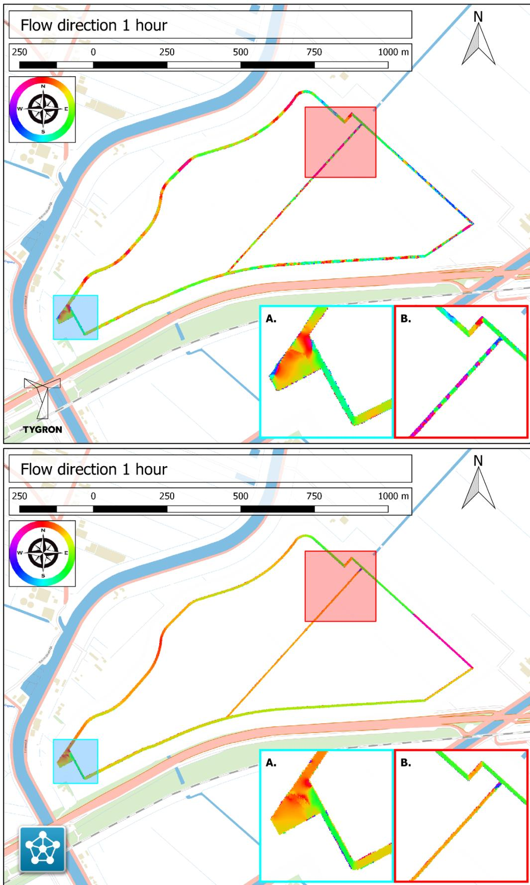
Figure A.7: Flow direction at 1 hour for Tygron (top) and Delft3D (bottom).
