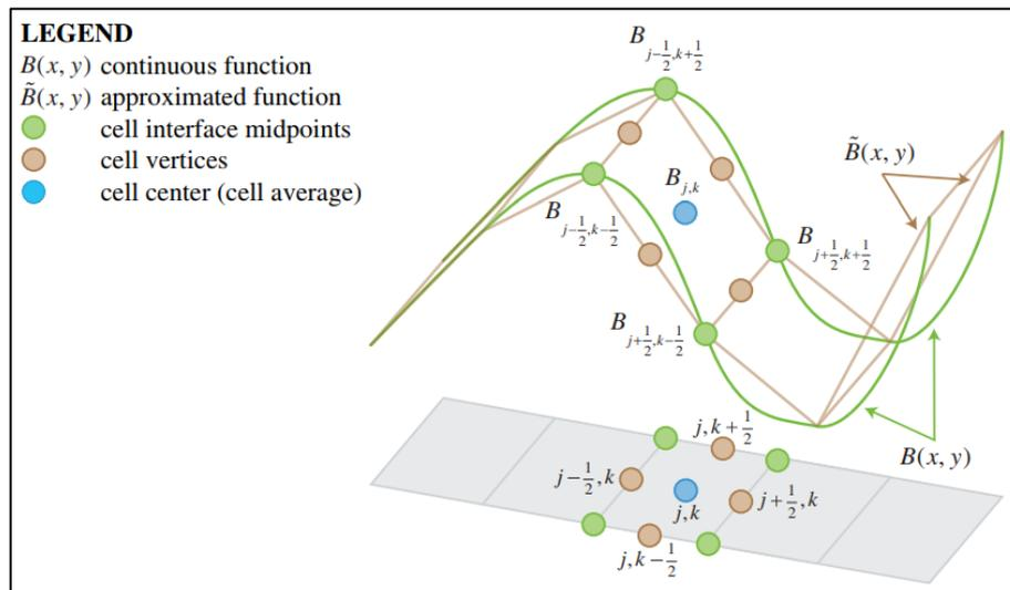
Figure 4.1: Discretization of surface height to computational grid in Tygron. Figure from (Tygron, 2019)
