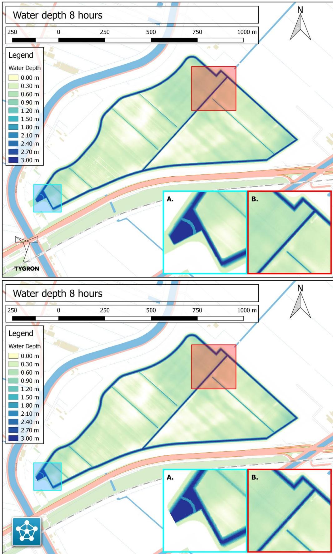
Figure A.3: Water depth at 8 hours for Tygron (top) and Delft3D (bottom).
