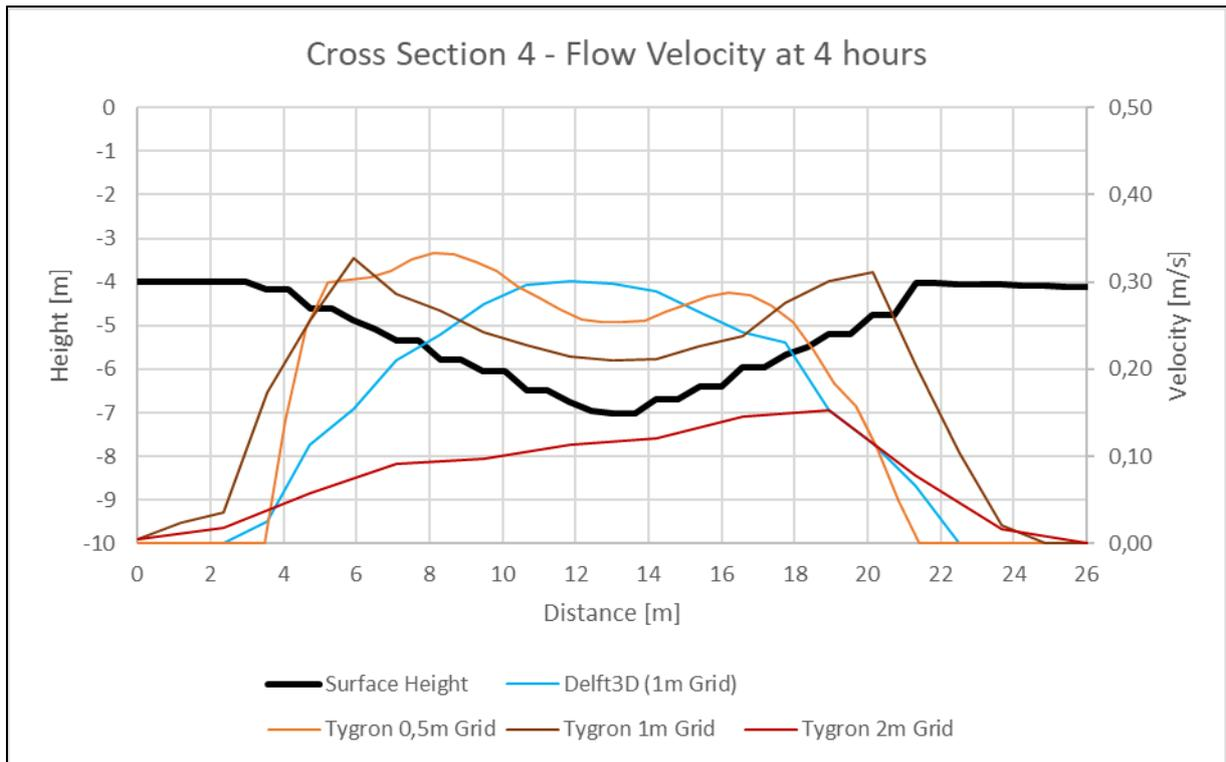
Figure B.4: Difference in flow velocity with different sized grids in Tygron.
