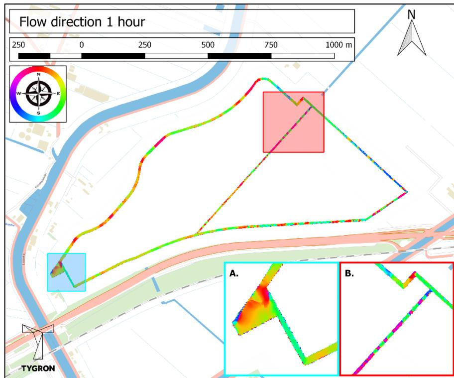
Figure 5.10: Flow direction at 1 hour for Tygron.
