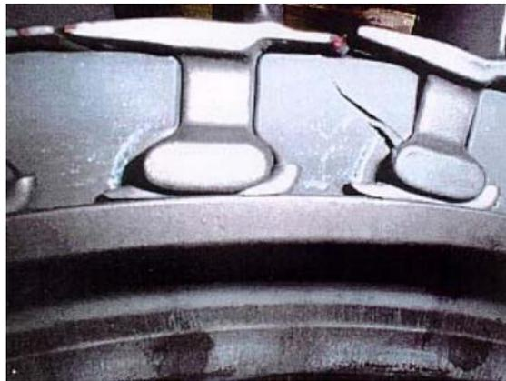
Figure 8 Crack initiated in rotor hub due to fretting[41]
