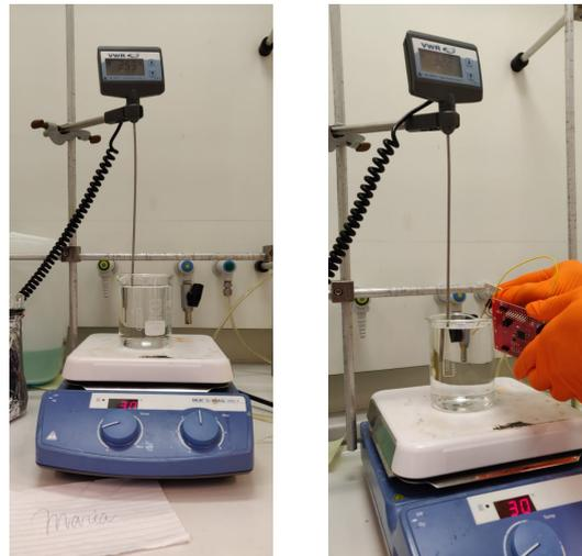
**Figure 5.12:** Test setup for temperature sensor calibration.
