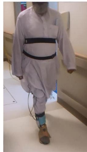
(b) SmartSox system based on Fiber Brag Grating (Najafi et al. (2017)).
