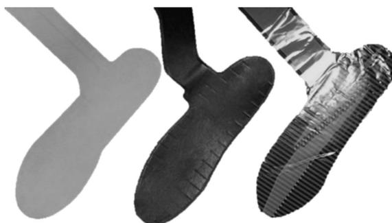
**Figure 4.1:** Designs of three insole systems: (from left to right) Pedar, Medilogic and Tekscan. (Adopted from Price et al. (2016))
