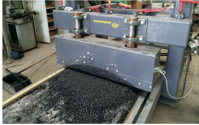
Figure 7: Oscillating screed test setup
