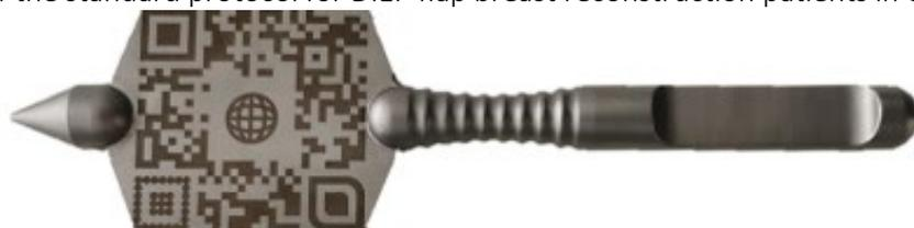
Figure 8: In-house designed stainless steel pointer with a laser engraved QR marker, used to indicate abdominal nevi on the patient to register the holographic anatomy into the patient.
