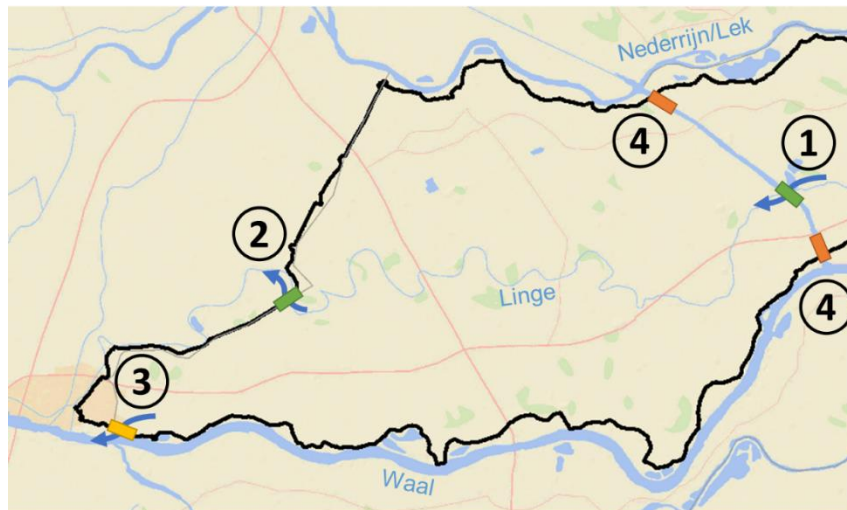
Figure 2-4: Locations of some the main hydraulic structures of dike ring 43: 1) Linge bypass sluice below the Amsterdam-Rhine Canal; 2) Linge discharge sluice in the Diefdijk; 3) Spill flow works at Dalem; 4) Shipping locks at the Amsterdam-Rhine Canal
