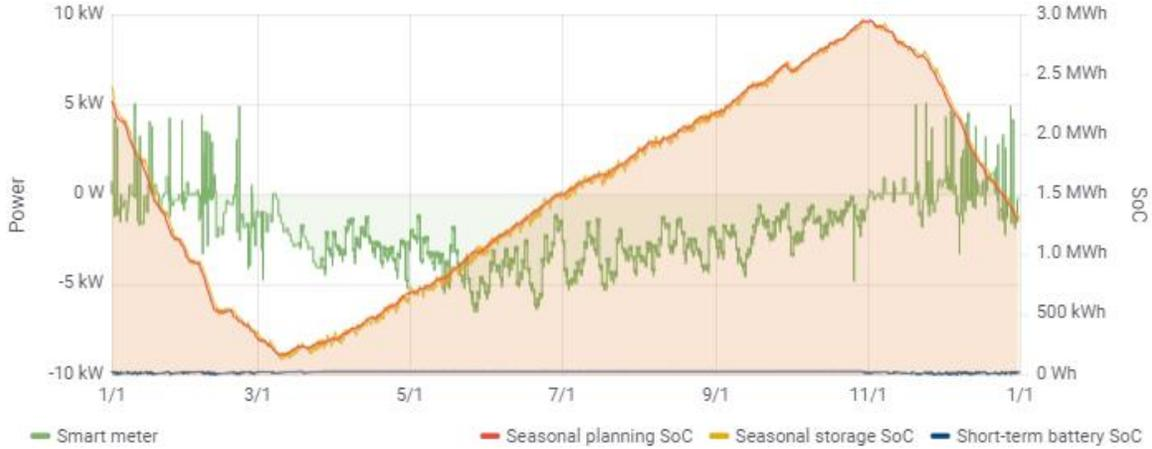
Figure 4-7 The simulation profiles of PSHBC-30-3000 with initial SoC set to 2.4 MWh
