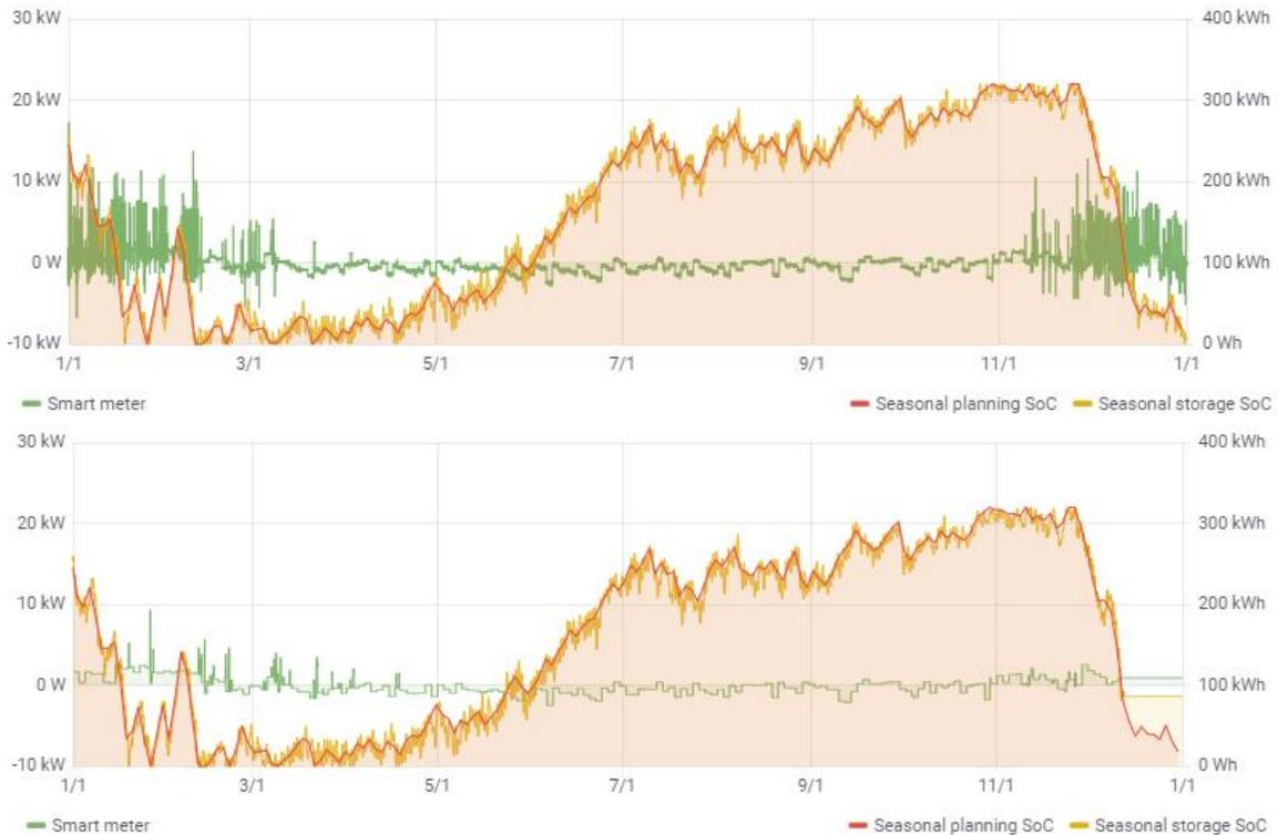
Figure 3-19 The comparison between the on (lower) and off (upper) of the balancing mode for solo seasonal storage with PS control algorithm
