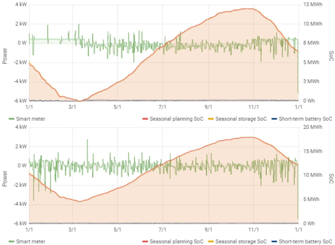
Figure 4-9 The comparison between the profile results of PSHBC-210-12000-ST (upper) and PSHBC-270-18000-ST (lower)
