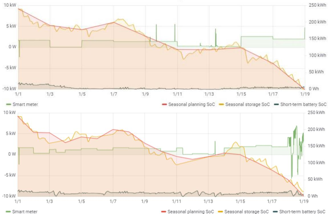
Figure 3-20 The comparison between the perfect realization of the seasonal target (upper) SoC and short-term rolling-horizon simulation method (lower) for hybrid storage system
