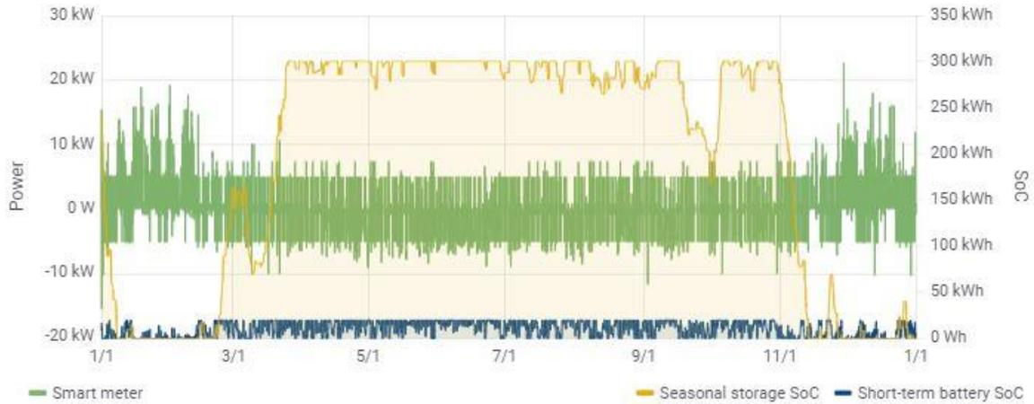
Figure 3-18 Control group – the hybrid storage system with no control
