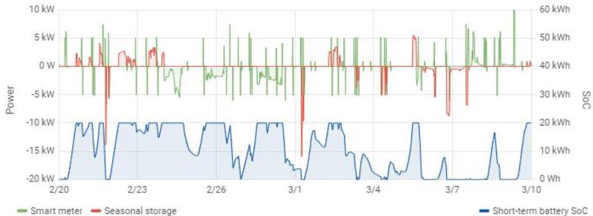
Figure 3-17 The operation of the hybrid storage system based on the on-off condition for no control
