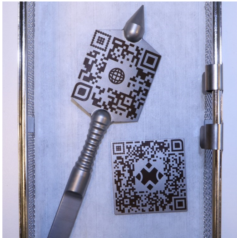
Figure 7 Stainless steel pointer with QR-code and reference QR-code.
