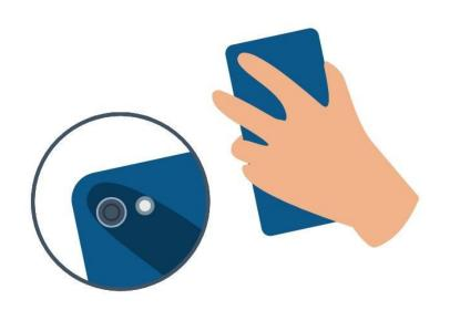
The flash light makes your veins visible for the camera., so we are able to analyze your pulse waves.
