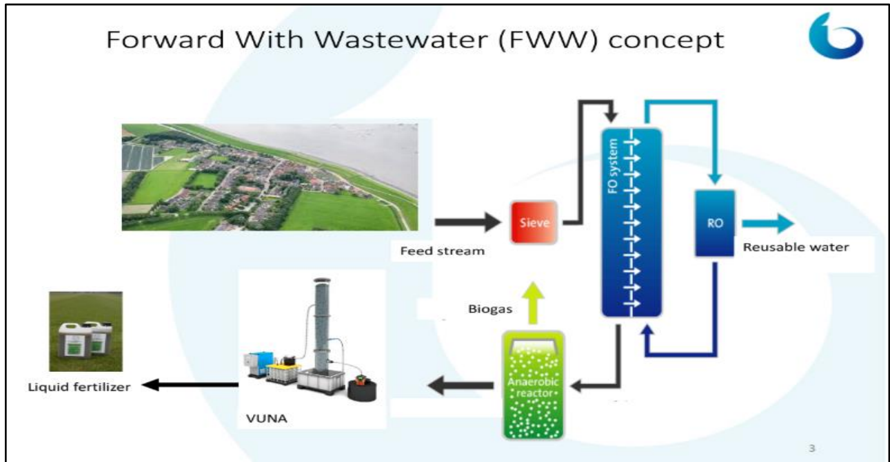
Figure 11. Core project with sieving as pre-treatment, FO and RO as primary treatment for reusable drinking water provision, anaerobic digestion with high rated anaerobic reactors which provides biogas. VUNA technology finally is applied for the production of liquid fertilizer.
