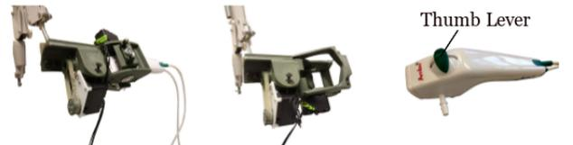
Fig. 5: Robot controller with Ambu endoscope (left), without the endoscope (center) and Ambu<sup>®</sup> aScope<sup>™</sup> 3 Regular (right) [5]
