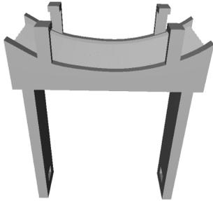
Fig. 8: New design of the pressor of the thumb lever of endoscope.
