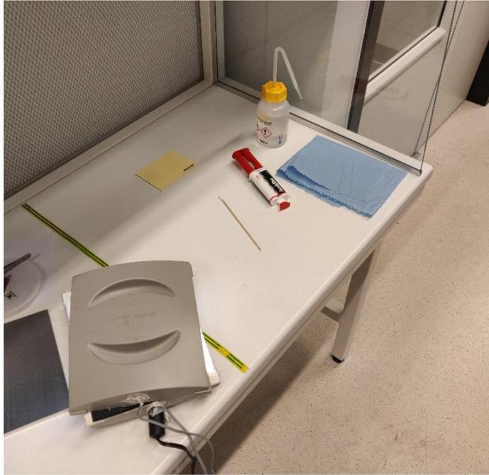
Appendix: Figure (7) - The tools needed for glueing: epoxy, alcohol, a piece of paper, a towel and wooden sticks. Optionally the chips could be placed in a lamp for better alignment with the inlets.
