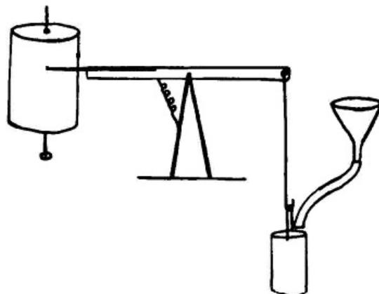
**Figure 2.2:** Design for first uroflowmeter by Willard M. Drake Jr. in 1946. From left to right the separate parts are a kymograph, a spring loaded balance with a writing arm, a fluid container and a collection funnel. Adapted from Chancellor (1998) [9].
