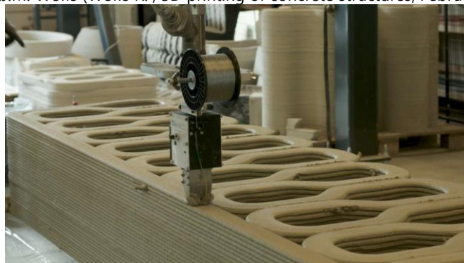
Figure 1.2: Example of 3D concrete printing (Bos, Wolfs, Ahmed, & Salet, August 2016)
