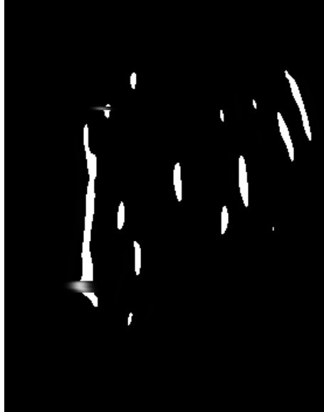
Figure 2.7: LoG filtered ultrasound image slice pre-filtered with a 1-dimensional Gaussian blur
