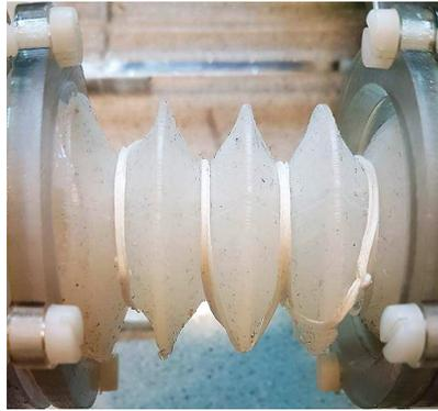
**Figure 2.10:** The improved SI actuator, which is shorter and wrapped by a strip.
