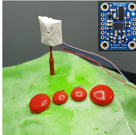
**Figure 3.2:** The IMU (at the top-right of the figure) is attached to a plastic needle which is inserted in the latex skin and liver phantom.
