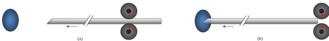
**Figure 4.3:** Concept I applied to the opposing rollers principle (a) during insertion, (b) once the desired depth is reached.
