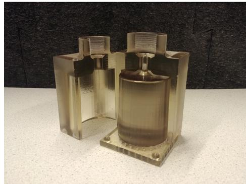
(b) Membrane mould, in upside down position
