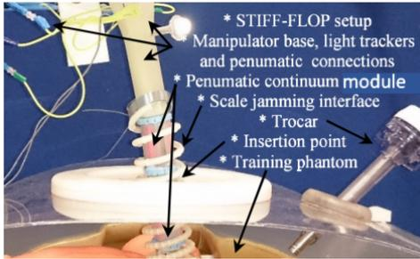
Figure 5: Scale jamming on STIFF-FLOP module. Spring made from smaller section which have the edges on an angle in a scale pattern.[3]
