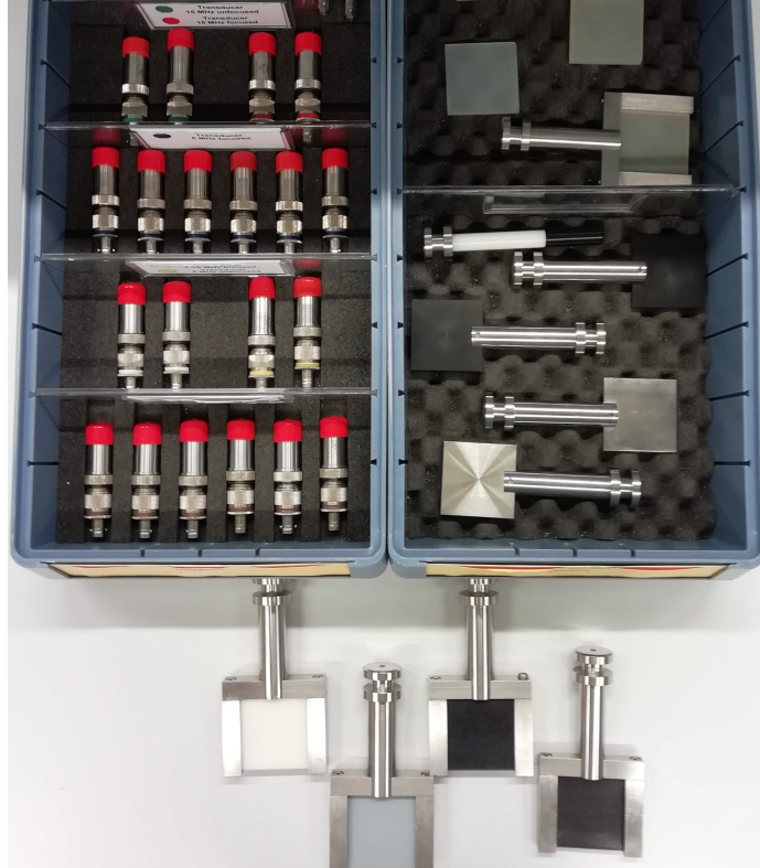
Figure F.2: Photograph of ultrasound probes and clamps with samples.
