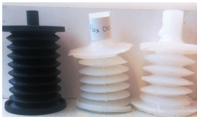
Figure 11: The three different actuators. On the left is the 3D printed actuator, in the middle is the Ecoflex 10 actuator and on the right is the Ecoflex 50 actuator
