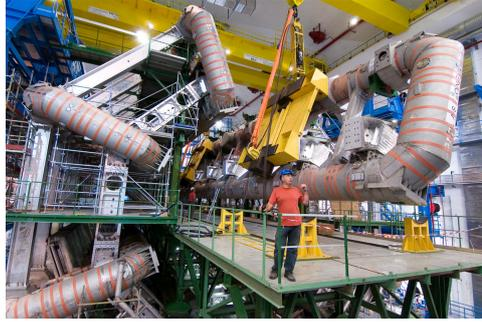
FIGURE 3.4: The ATLAS Barrel Toroid magnet [38]
