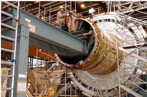
FIGURE 3.2: ATLAS Central Solenoid magnet [38]
