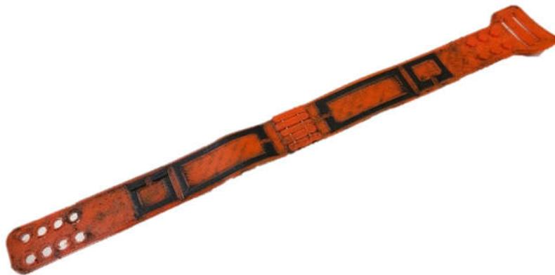
*Figure 1 FSS Band manufactured with flexible TPU, conductive (Black) dielectric (Orange).*
