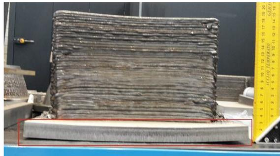
Figure 2.1: Distortions in a product manufactured by WAAM within Tecnia (source: internal Tecnia documentation)
