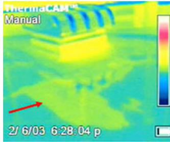
Figure 6: Roof Viewed Through Thermal Imaging [3]
