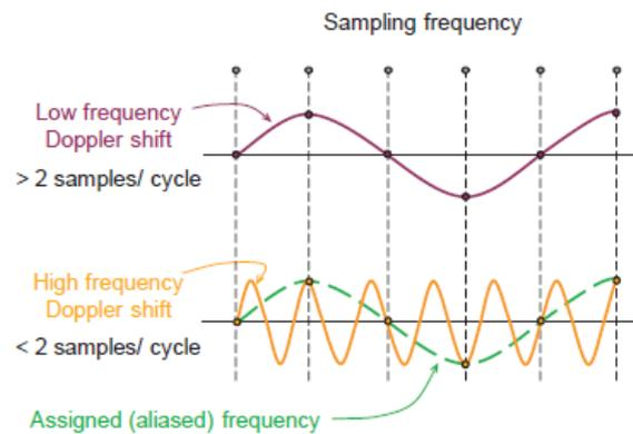
Figure 9 Aliasing during Pulsed Wave Doppler US.[24]
