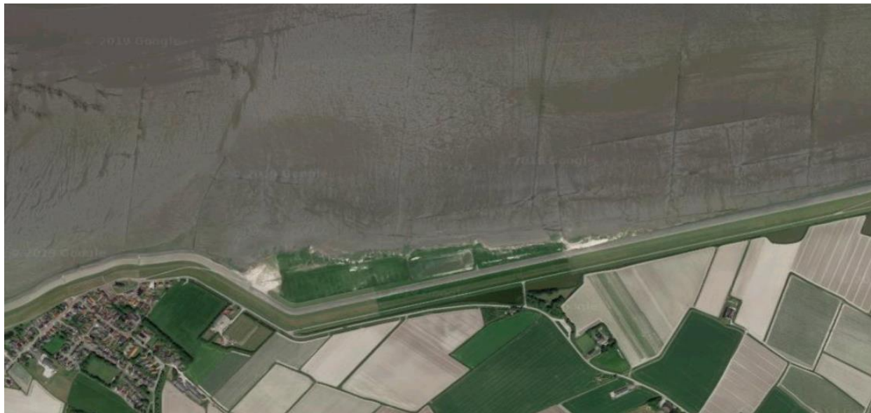
Figure 3. Satellite image of the eroding salt marsh of the study area, near Wierum. Remains of the old sedimentation fields and groyne can still be observed on the tidal flat.
