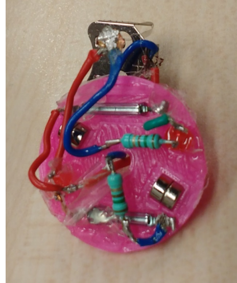
Figure 4.16: The printed PCB mock-up used to test the sensing principle with a battery in series with a reed switch, LED and resistor (two reed switches etc.).
