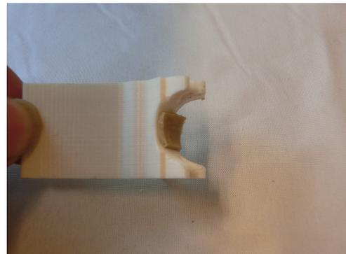
Figure 5.6: **The left locking gear**
