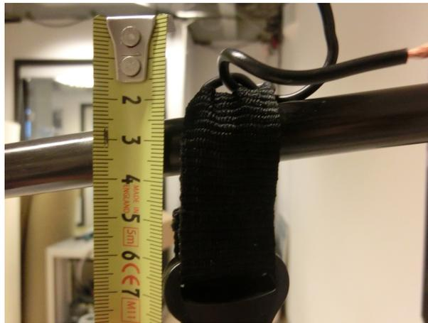
Figure 4.1: Measuring the bending of the mechanism when applying a force of 30 N at 0.40 m from the wall
