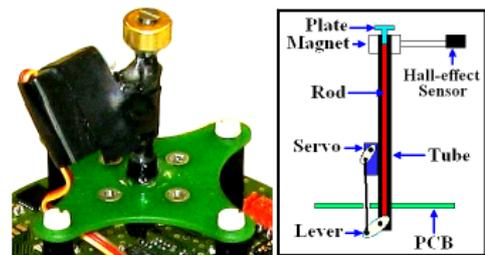
Figure 1.5: Attacher/Detacher mechanism using a magnet [6]
