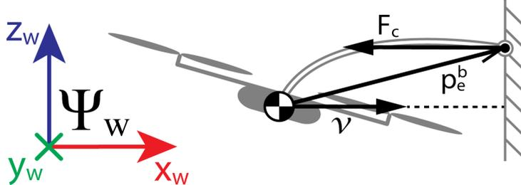
Figure 1.2: A Schematic overview of the forces acting on a drone with a manipulator while touching a wall.  $F_c$  being the reaction force of the wall on the end-effector and  $P_e^b$  being the position of the end-effector [3]
