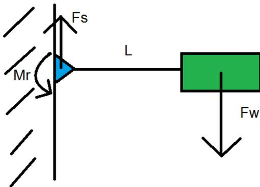
Figure 3.2: Initial force and moment calculations
