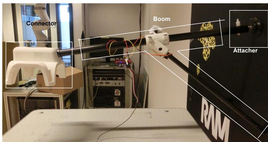
Figure 3.1: An overview of the different parts of the prototype
