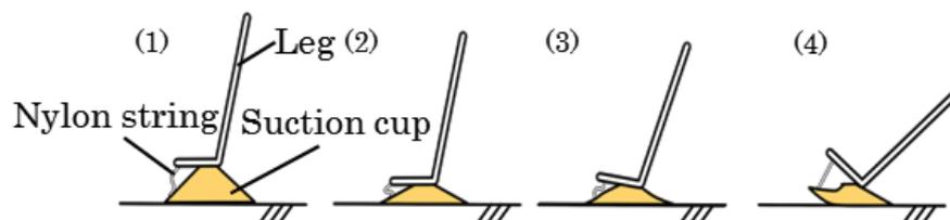
Figure 1.8: The detaching of the passive suction cup [9]
