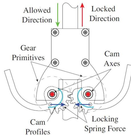
Figure 5.5: **The locking mechanism [3]**
