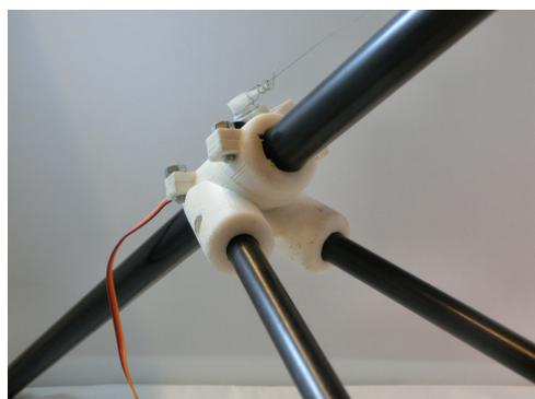
Figure 3.5: **The support connector**
