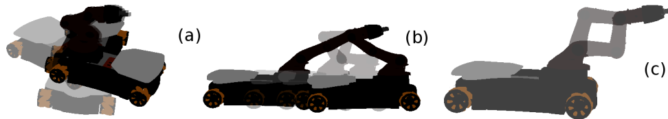
Figure 4.2: Rendition of the three redundancy parameters: (a) is \rho_1 , (b) is \rho_2 , (c) is \rho_3 (Sharma et al., 2012)
