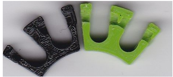
(b) Part of wheel frame printed in ABS (black) and PLA (green), showing that PLA prints sharp edges more accurate than ABS.
