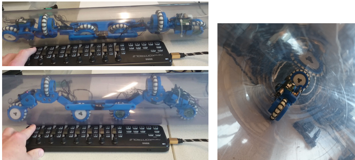
Figure 7.1.: Test setup with the robot inside a pipe with an inner diameter of 85 mm (top) and one with an inner diameter of 120 mm (bottom & right). During the test the robot is controlled using the controller panel as shown in front of the pipes.
