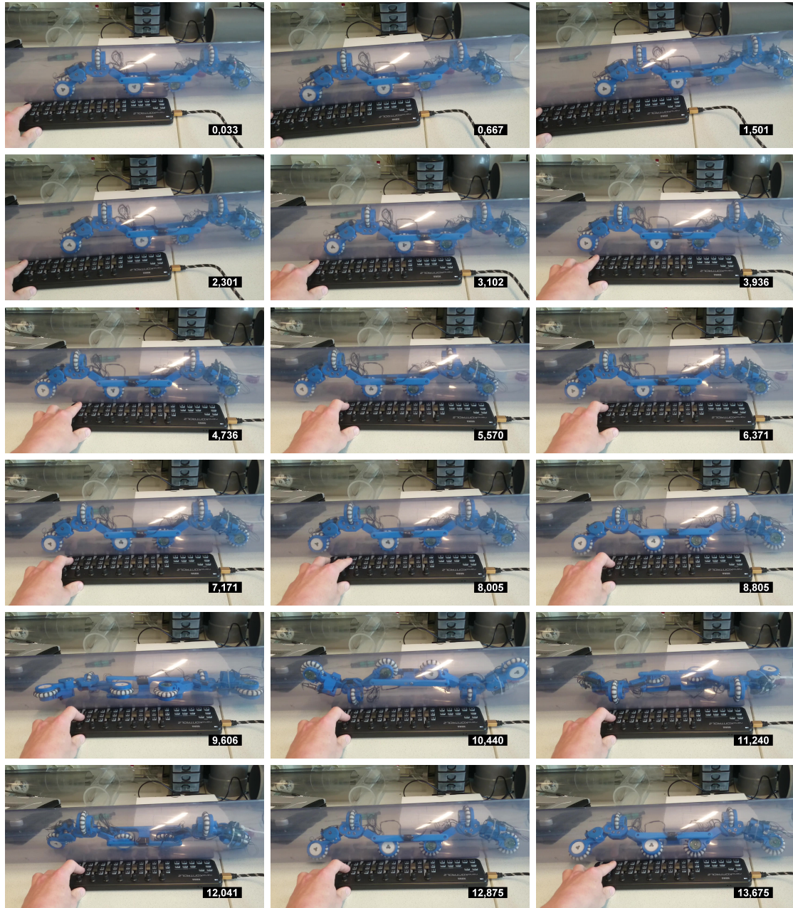
Figure C.2.: Translational and rotational motion of the robot inside a 120 mm pipe.
