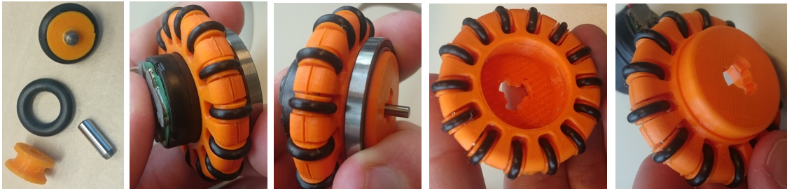
Figure 2.8.: Realized roller and wheel, also shown with motor and bearing.
