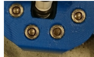
(d) Bearings and pins at the outside of the body, going around the omniwheel.
