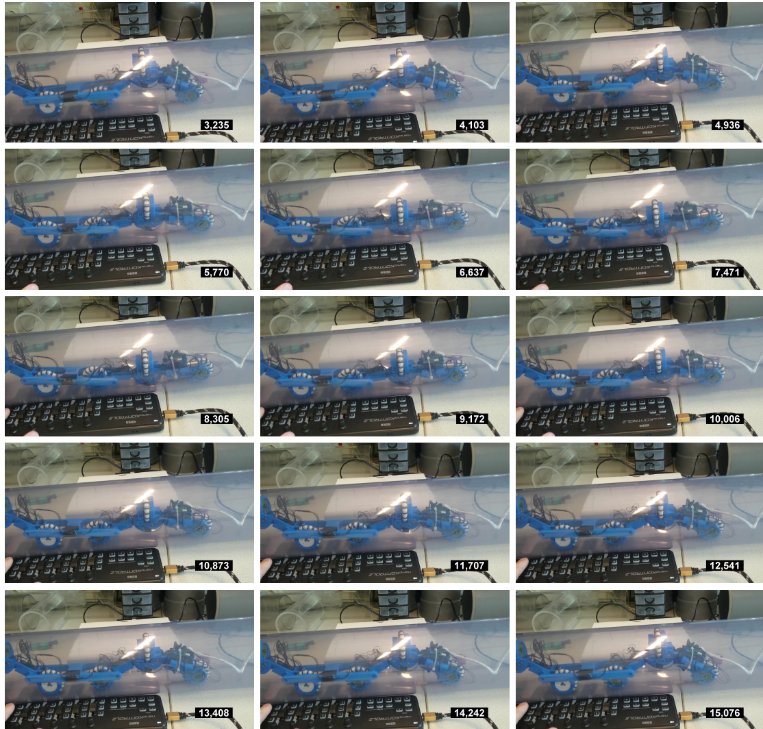
Figure C.3.: Unclamp and re-clamp of the robot inside a 120 mm pipe.
