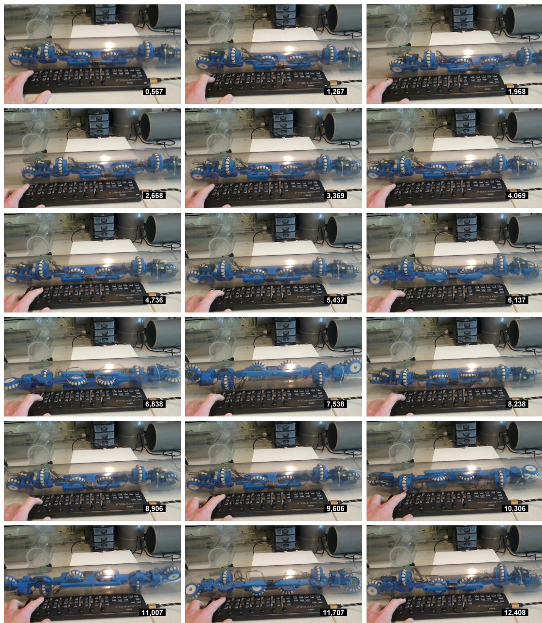
Figure C.1.: Translational and rotational motion of the robot inside a 85 mm pipe.
