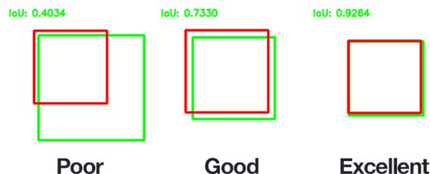
Figure 4.10: A visual representation of the intersection over union. The green box represents the true area (ground truth) and the red box represents the predicted area. [16]
