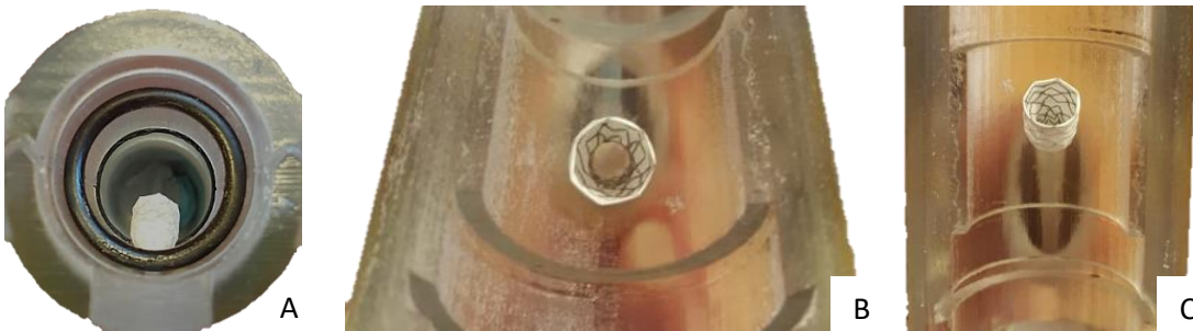
Figure 2: BeGraft balloon expandable covered stent flared in the 45 degrees branch of the phantom model. A) top view of the phantom model, B) look through view of the BECS, C) side view of the BECS
