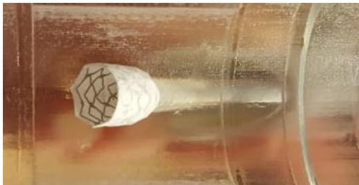
Figure 3: A flared BECS in an in vitro aorta phantom model
