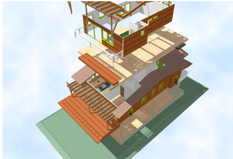
Figure 8: Although not in the strict sense axonometric, this building is rendered with a greatly reduced perspective effect. The floors are separated, forming an 'exploded' view. [10]
