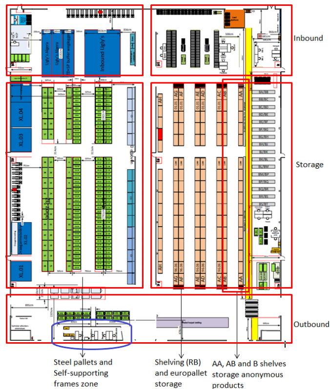
Figure 5-1: Floor map incl. location new Lean-Lifts
