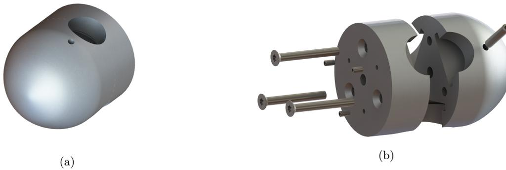
Figure 5.1: The assembled hub part(a) and an exploded view of all parts in the hub (b).
