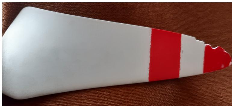
Figure 6.6: The chipped rotor blade.
