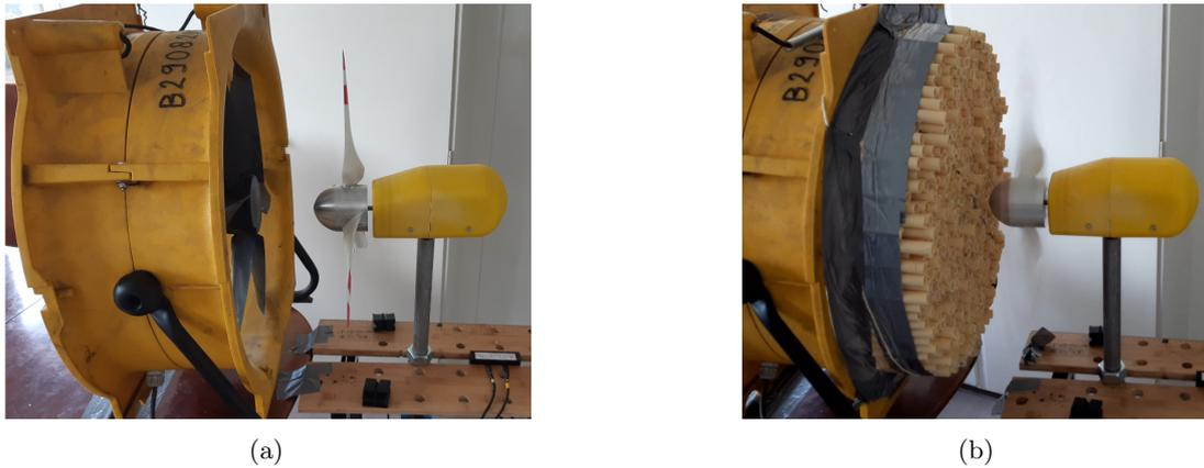
Figure 6.4: The test setup without the flow straightener (a), and the test setup with flow straightener (b).
