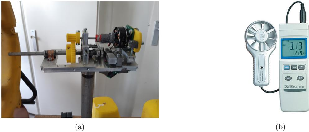
Figure 6.3: The sensors and gearing inside the nacelle for test 2 (a), and the anemometer used to determine the wind velocity (b).
