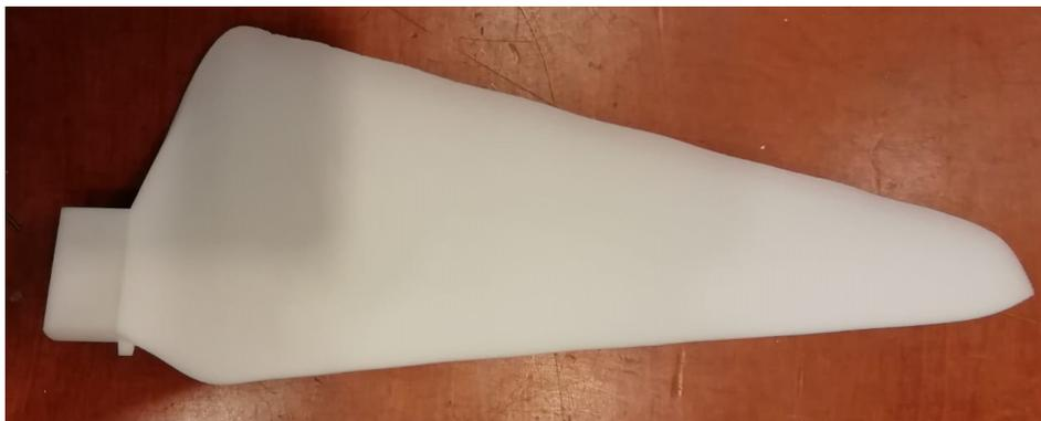
Figure 5.7: The first printing test of the designed blade.
