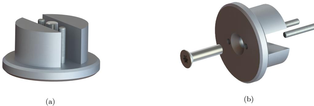
Figure 5.2: The assembled blade foot (a) and an exploded view of all parts in the blade foot (b).
