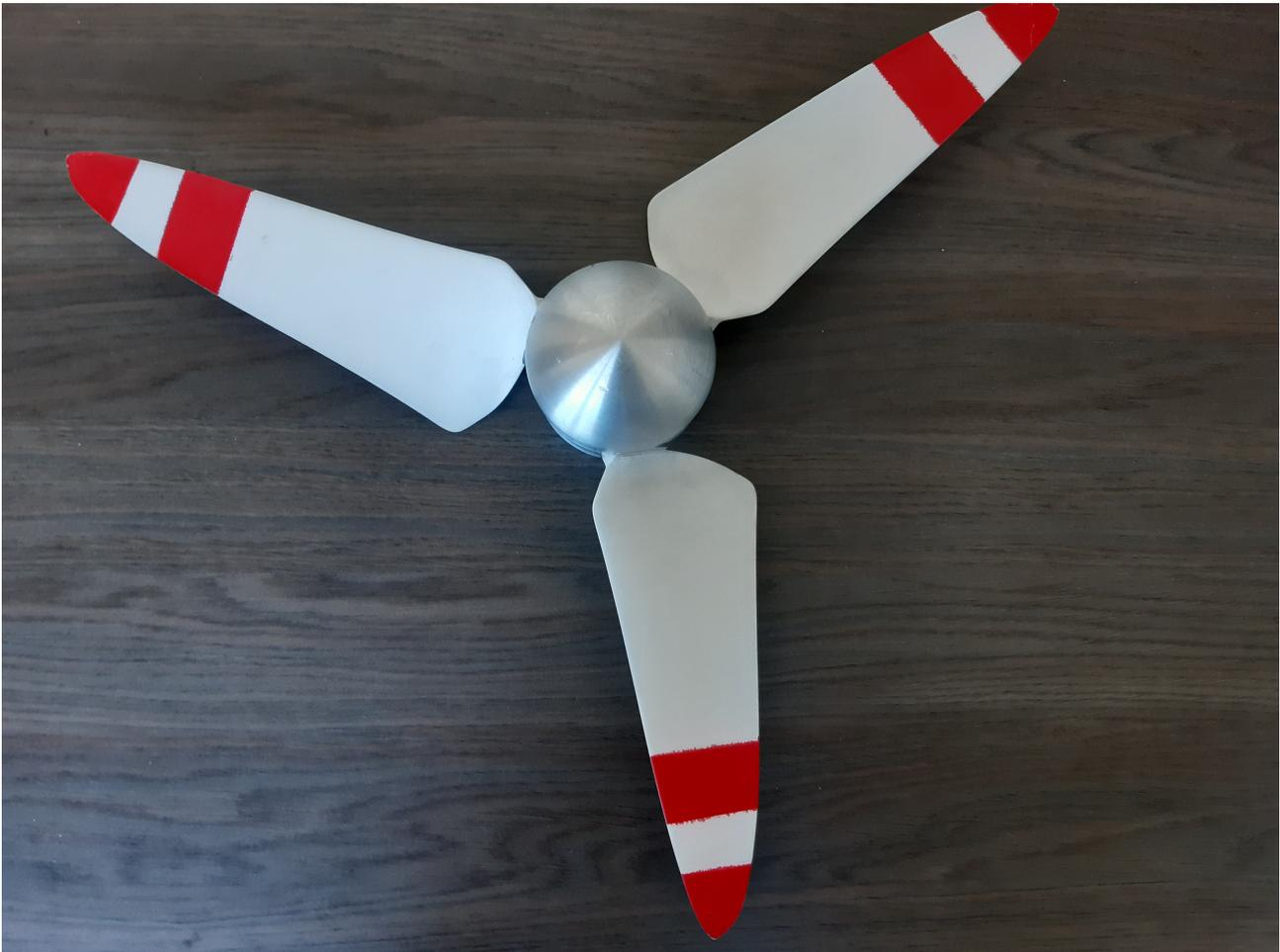
Figure 5.20: The assembled rotor.
