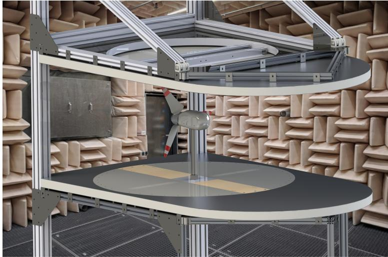
Figure 2.1: The wind turbine experiment setup in the UT wind turbine.
