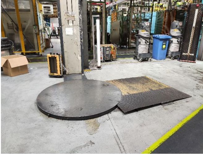
Figure 6.9. Fixed pallet foil wrapping place
