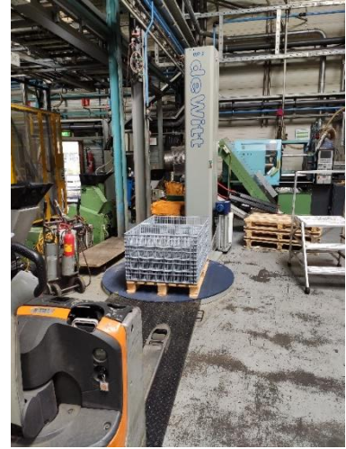
Figure 6.10. Flexible pallet foil wrapping
