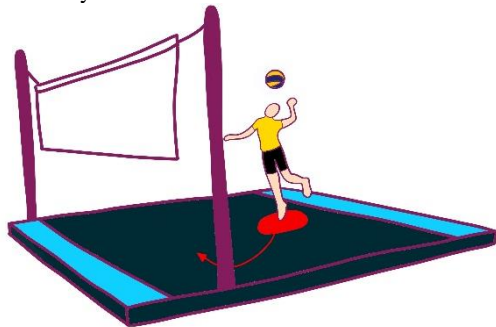
Figure 1-1 This illustration depicts the interactive LED floor set up as half a volleyball court. The red circle indicates the player's current location and the red arrow indicates the player's next move.
