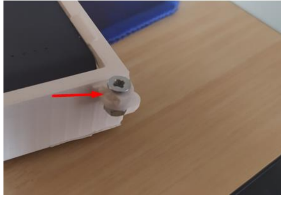
Figure 37: Connector component breaking as a result of the prioritizing tightness in the nuts and bolts. This is indicated by the red arrow.
