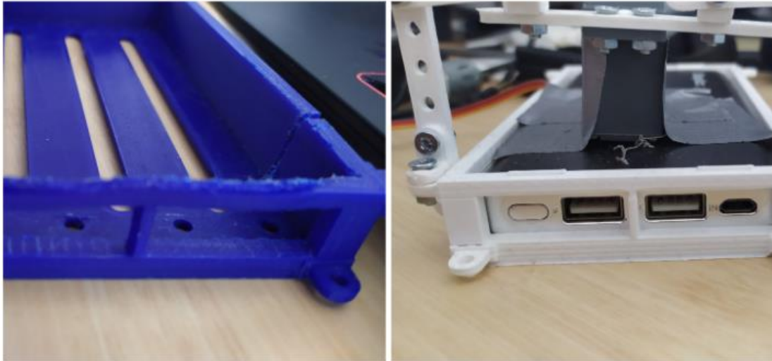
Figure 29: Models of the power bank base. The first version on the left showing how it had to be cut open and melted to make the power bank securely fit inside of it. The second version on the right showing it securely fitting and holding the powerbank in place, while also function as a base for the addition of other components.
